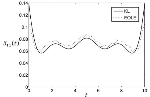
Figure 1. Point-wise variance error  $\delta_{11}(t)$  for the multivariate KL and EOLE methods with  $m = 6$ .
