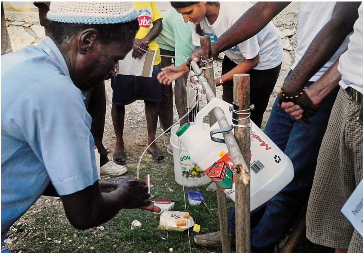
Fig. 77: Construction and test of a Tippy Tap for hand washing (Courtesy of Mariana Aramayo Donoso, 2013)
