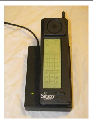
*Figure 9: The IBM Simon from 1994 is considered the first smartphone by some. [Source: https://commons.wikimedia.org/wiki/File:IBM\_SImon\_in\_charging\_station. png]*
