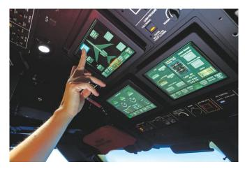
Figure 24: Due to easy integration, touchscreens will be integrated in a variety of places. This can lead to solutions that even require regular overhead use like this cockpit of a Gulfstream G500/G600. [Source: https://coeaerospace.com/cockpit-controls/]
