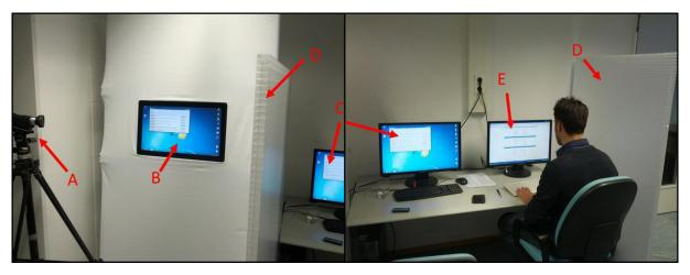
Figure 67: Participant in the usability lab during the stationary touchscreen study. Camera (A), touchscreen (B), experimenter's control PC (C), screen (D), questionnaire PC (E)
