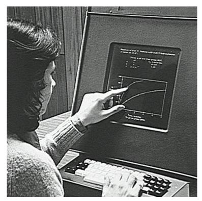
Figure 6: The University of Illinois' PLATO IV computer system was the first widely deployed computer with optical touchscreen. [Source: https://archives.library. illinois.edu/erec/University%20Archives/1505050/BrownBag/BBPlatoIV.htm]
