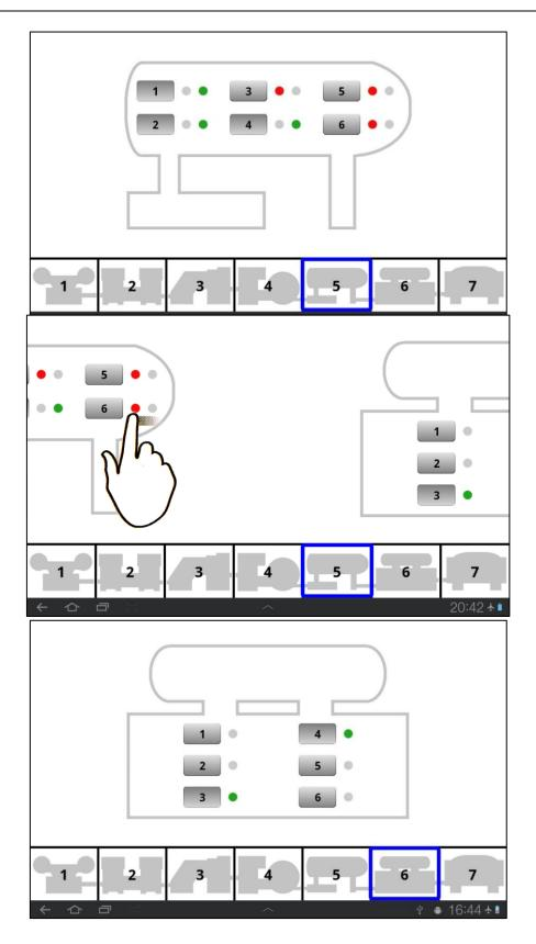
Figure 62: Implementation of the Page-Flip variant. A drag to the left switches from machine #5 to #6
