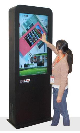
Figure 23: Touchscreen systems may lead to a variety of different postures for giving input. This touchscreen stand shows the common problem that users have to hold out their arm for some time when interacting. Moreover, this system will even force smaller users to reach overhead. [Source: http://www.senpallcd.com]
