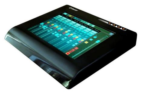
Figure 12: The Lemur music controller was the first commercially available touchscreen device that supported unlimited multi-touch. [Source: http://www.jazzmutant.com/]
