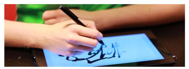
Figure 22: Palm recognition, also known as palm rejection, allows users to rest their hands on a horizontal touchscreen in an attempt to reduce strain on the arms and improve input precision. It is mostly integrated in touchscreen systems that can be controlled with a stylus. [Source: https://www.robertxiao.ca/research/]
