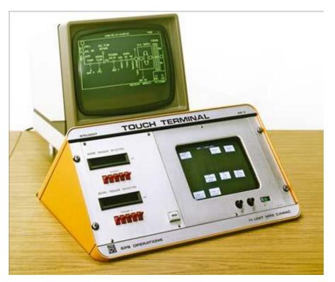
Figure 5: The first transparent, capacitive touchscreens (bottom) were developed and used at CERN. [Source: https://cerncourier.com/the-first-capacitative-touch-screens-at-cern/]
