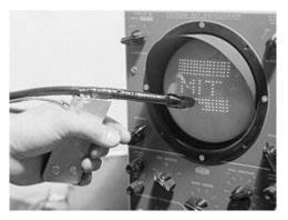
Figure 3: MIT's Whirlwind computer was the first to allow for direct interaction on the screen using a light pen. [Source: https://history-computer.com/ModernComputer/ Electronic/Whirlwind.html]
