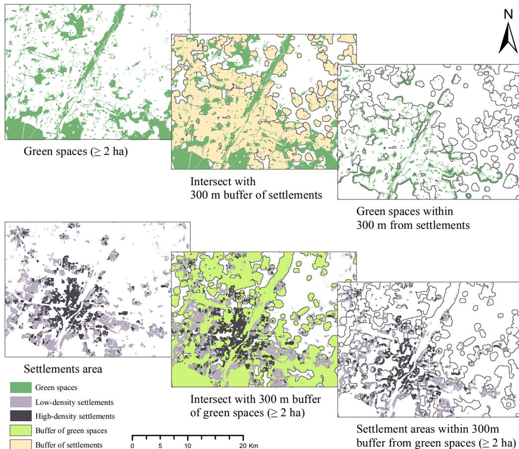
**Figure 3.10** Processes of the spatial calculation in ArcGIS.
