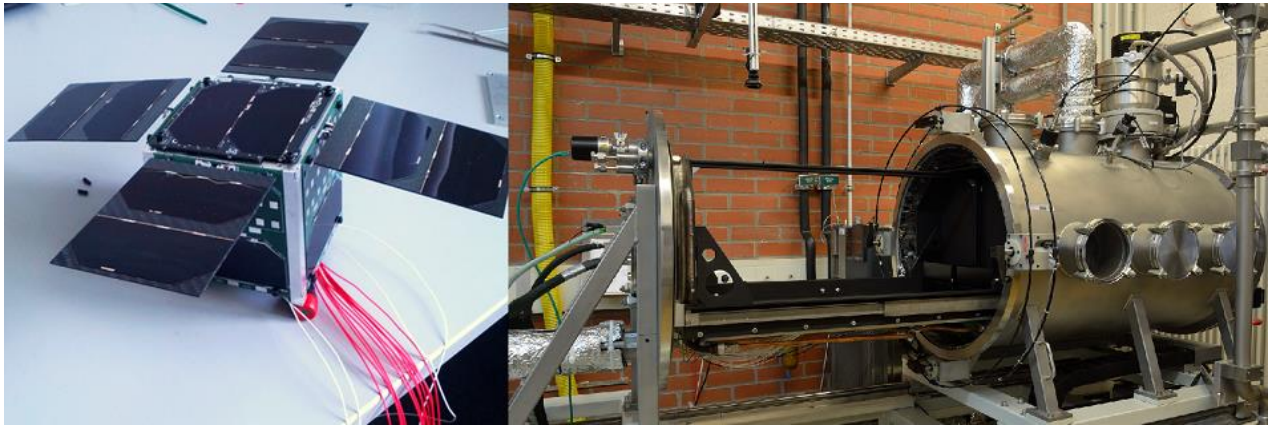
Figure 4-89: Thermal Prototype of MOVE-II and TVAC of LRT.
