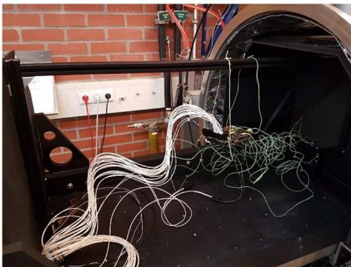
Figure 4-90: Subsystem-level test in the TVAC (left) and System Level testing of the MOVE-II FM (right). Image Source: [288].
