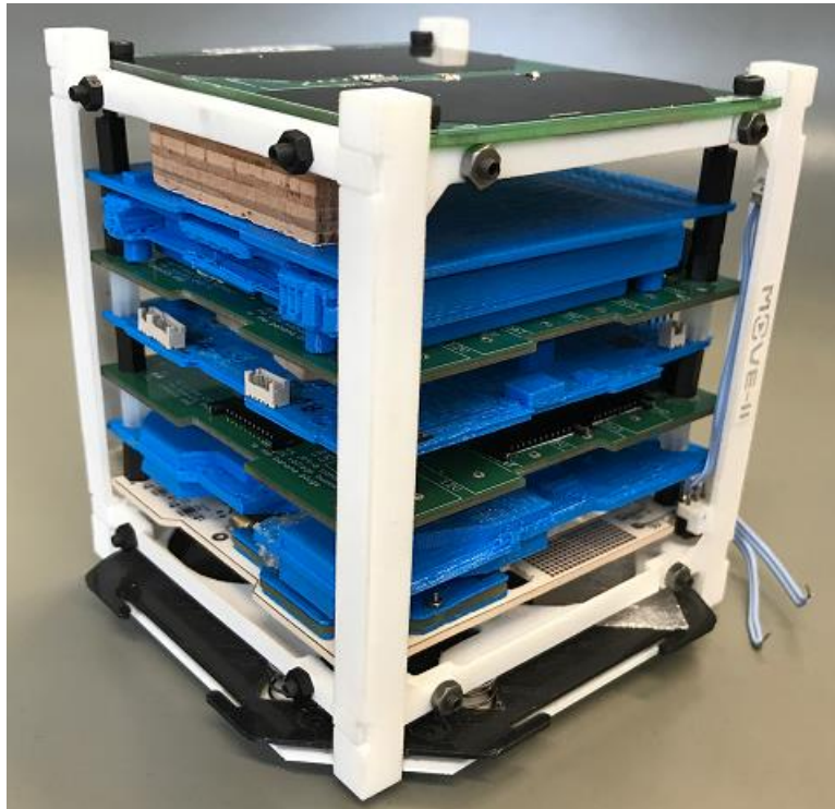
Figure 4-93: 3D Printed Prototype of MOVE-II
