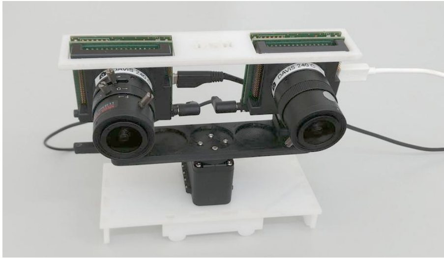
Figure 1.1: A stereo vision setup consisting of two event-based vision sensors in a rigid frame
