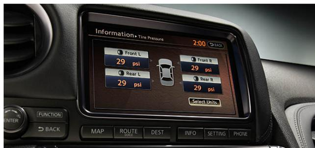
Figure 2-7.: Information about tire pressure of the vehicle’s tires displayed in the 2016 Nissan GT-R<sup>7</sup>.
