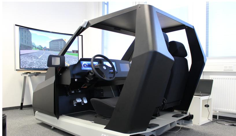
Figure 8-2.: The driving simulator mock-up used in this user study.
