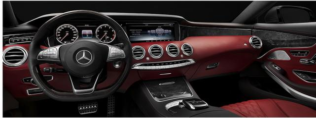
Figure 2-3.: The cockpit of the S-class model BR222 from Mercedes-Benz includes a free-programmable cluster display and head-unit display. In addition, information can be shown on a head-up display or rear view and side mirrors<sup>3</sup>.
