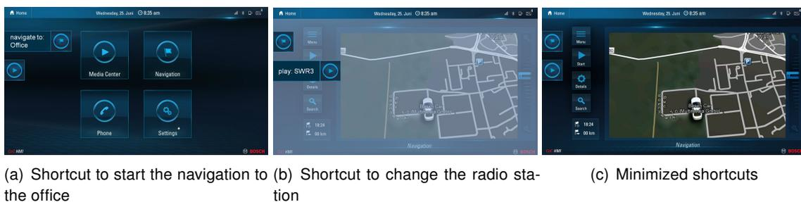
Figure 6-7.: A second variant of the support level US is realized by displaying the shortcuts in form of notifications. The notifications are moving into the screen from the left side. If the driver has recognized them but is looking away, they will be minimized automatically. In addition they can be minimized and maximized by clicking on the icon of the application.
