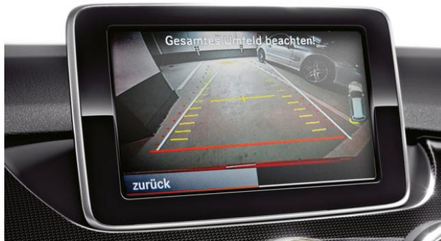
Figure 2-9.: The picture of a rear-view camera, which belongs to an electronic parking assistance is shown on the head unit display of a Mercedes-Benz<sup>9</sup>.
