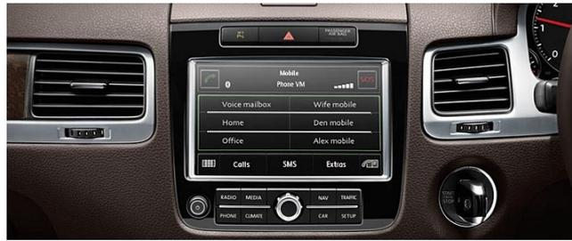
Figure 2-10.: The main screen of a phone application of a VW infotainment system shows available functions like speed dial options of the connected phone<sup>10</sup>.
