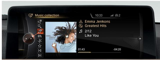
Figure 2-6.: The media screen of the BMW ConnectedDrive infotainment system shows the title of the currently played song, which is located on another device<sup>6</sup>.
