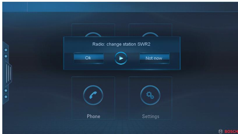
Figure 7-6.: Variant A - Recommendations are given in form of pop up messages, which need to be accepted or rejected by the user (User Approval).
