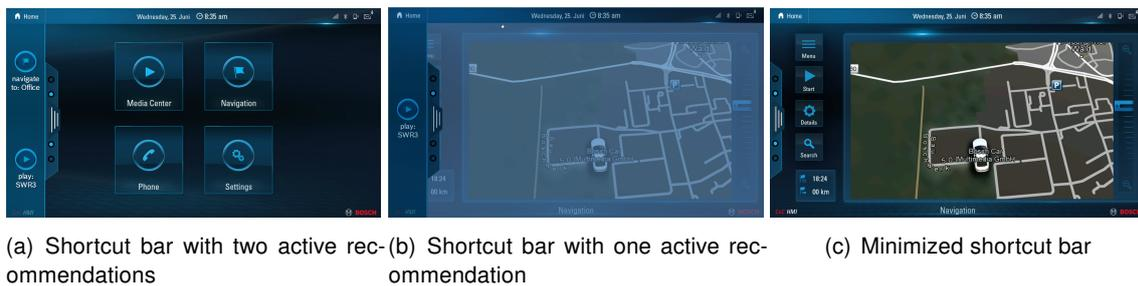
Figure 6-6.: One variant to realize the support level US is a shortcut menu bar, which is shown at the left side of the screen. The menu bar can be minimized and maximized by an indicator shown in the middle of the bar. Up to four recommendations can be displayed. The number of displayed recommendations is indicated by four dots even when the menu bar is minimized.
