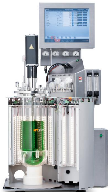
Figure 13: The benchtop Labfors 5 Lux photobioreactor system by Infors. (Infors AG, 2017)
