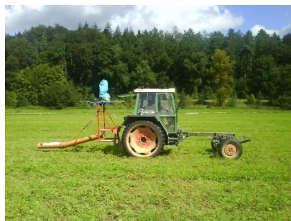
Figure 2. Mounting of the EM38 on a metal-free sledge pulled by a tractor (constructed after Corwin and Lesch [7]).
