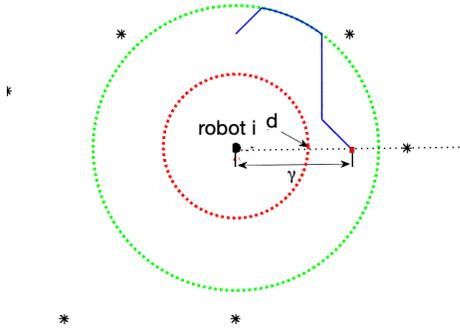
Fig. 5: The detecting process. Green dashed circle is robot  $i$ 's sensor range. Red dashed circle is direction ring of robot  $i$ . Black dot represents the robot  $i$ . Star dot represent other robots in  $N_i$ . The black dashed line is the ray  $\overrightarrow{p_i p_d}$ . Red point is the  $q$  who satisfies the stop criterion. The blue solid line is part of the dominating region boundary.
