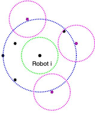
Fig. 3: The identification of neighbor set  $N_i$ . The visibility range and the communication range of robot  $i$  are denoted by the green and blue circles, respectively. The robots marked in magenta are identified not the neighbours of robot  $i$ .
