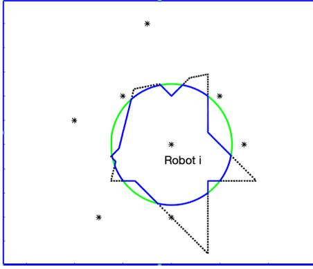
Fig. 2: The dominating region in order 2 Voronoi partition of robot  $i$  with limited sensing range. The robots are denoted by stars. The dashed line is the dominating region of  $n_i$  in order 2 Voronoi partition without range limitation. The green circle indicates the sensing range. The blue solid line is the final boundary of the dominating region  $D_i^k$ .
