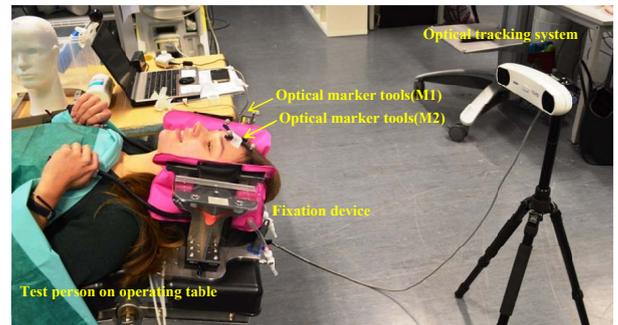
Fig. 4. The experimental setup for movement evaluation. Optical marker tools M1 is fixed on the head fixation, and M2 is mounted on the experimenter.
