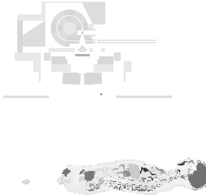
Figure 5.12: MCNPX cross section plot of the Clinac and ICRP phantom in the y - z -plane (in-plane) for a 0^{\circ} gantry angle. Different materials are indicated by different grey values. Some structures, e.g. vacuum window and mirror, are not displayed as their thickness is below the resolution of the picture.
