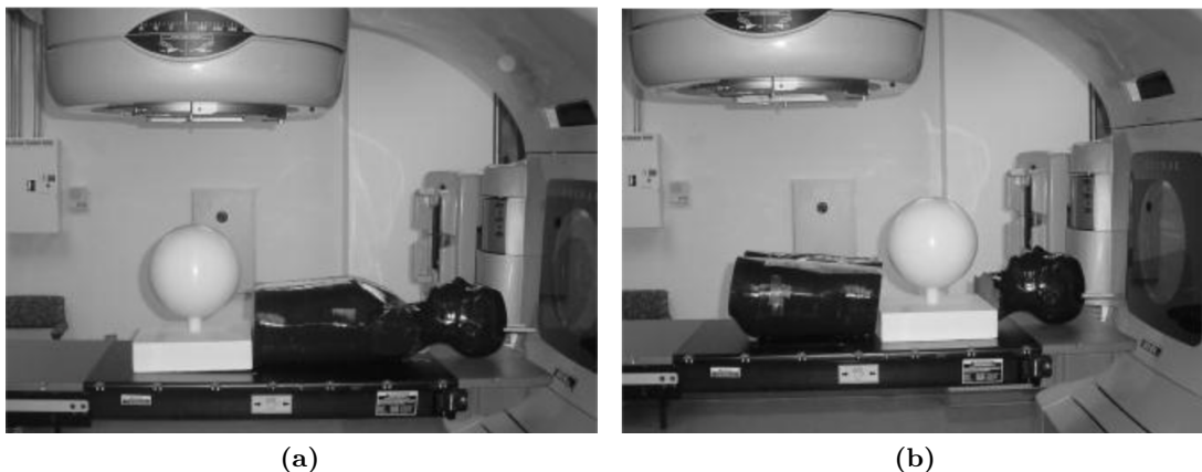
Figure 7.5: Setups for in- and out-of-field measurements with a 10 in. Bonner sphere carried out by Howell et al. [How06]. (a) at the isocenter and (b) at 40 cm superior to isocenter. Based on those two measurements Howell derived the neutron equivalent doses for all organs. The values are reported in table 7.1.
