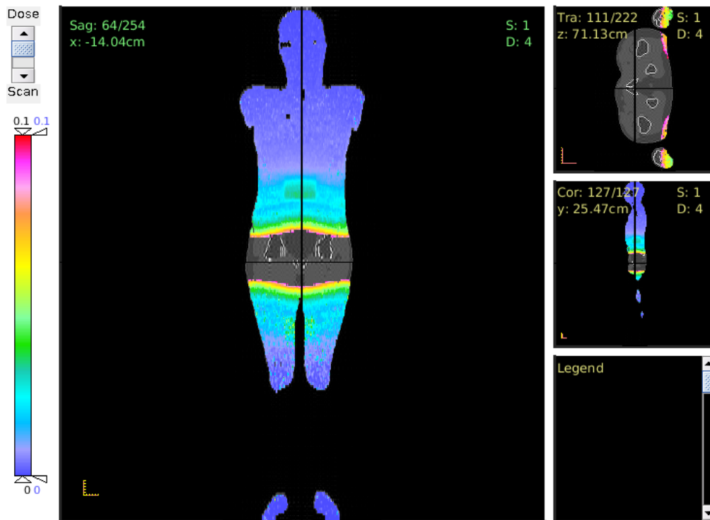
Figure 6.7: Photon absorbed dose distribution of the 3D-CRT treatment in the coronal phantom plane. The dose values are limited to a maximal value of 0.1 Gy in order to provide a better contrast. The unit of the color code is [Gy].
