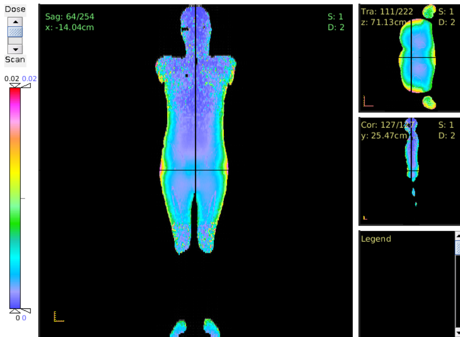
Figure 7.2: Neutron dose equivalent distribution of the 3D-CRT treatment in the coronal phantom plane. The unit of the color code is [Sv].
