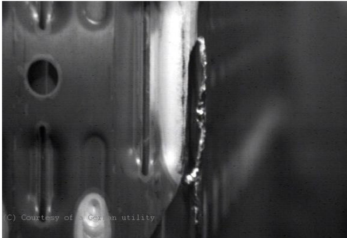
(a) Photograph of grid corner fretting damage (Spykman and Pattberg, 2014).
