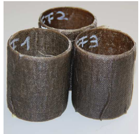
Fig. 4: Specimen Tubes made of Flax Prepreg Material
