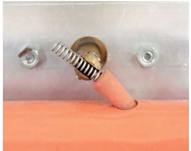
Fig. 5 The papilla is inserted into the opening of the duodenum and fixed to the mount by gently pressing its metal coil into the groove of the mount. The metal coil serves for grounding the papilla via the mount connected to a socket at the back. When the carriage is closed, the coil leads instruments inserted into the papilla into the bile duct. This can be viewed in the window of the simulator.
