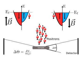
**Figure 5.** Schematic picture of spin-polarized 2D-ACAR. In electron-positron annihilation the singlet configuration is preferred for majority or minority spin electrons if the magnetization of the sample is parallel or anti-parallel to the emission direction of the positrons.
