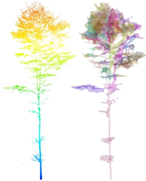
Figure 11.: (l) Original point cloud and (r) individual branch space occupation estimation achieved by combining skeleton data with \alpha -shapes of a kd-tree based nearest-neighbor assignment for a European beech test tree (Bayer et al. 2013).
