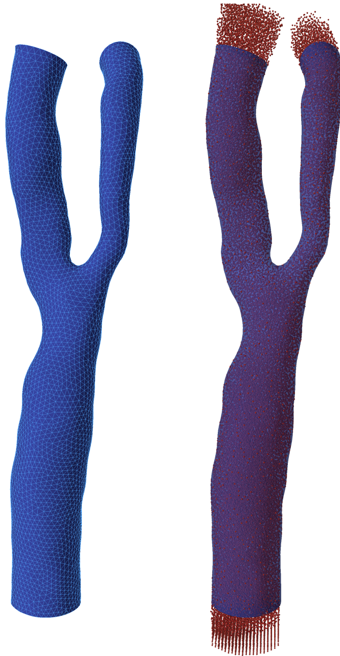
Figure 5.7: Patient-specific modeling of blood flow using SPH. On left, tessellated three-dimensional surface of the CAB is shown. Surface data can be used to simulation flow in arbitrary geometries. On right, initialized SPH domain to model flow in CAB is shown. Inlet and outlet particle buffers extend the computational domain beyond those of the geometry.
