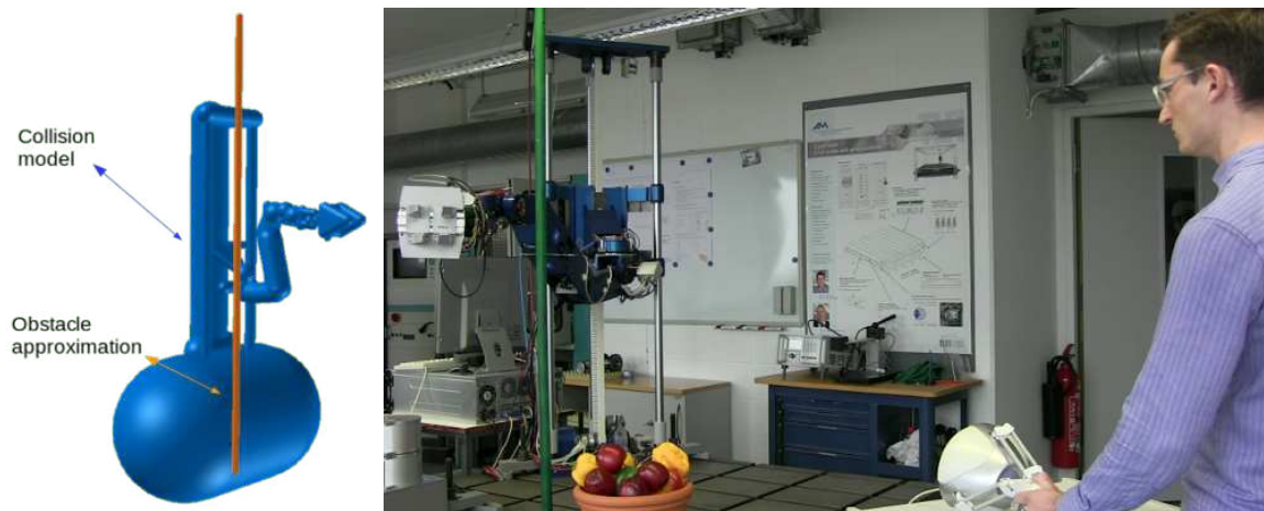
Figure 4.15: Obstacle Avoidance with robot manipulators. Left: both the robot and the obstacles can be modeled using SSVs. Right: the robot is controlled via tele-operation but adapts its path to avoid a vertical object.
