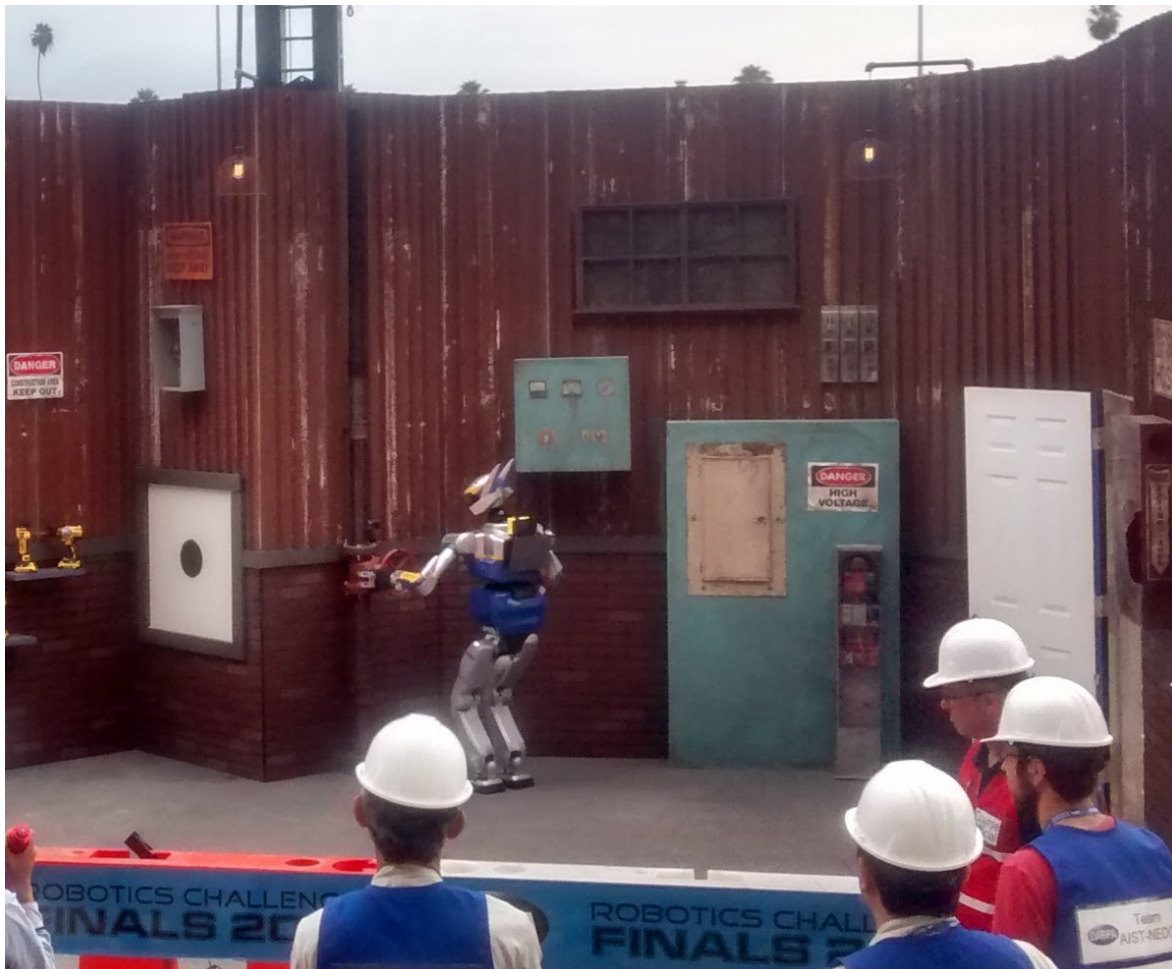
Figure 1.1: The DARPA Robotics Challenge tested robots with tasks inspired by the Fukushima disaster. In this picture, the Japanese robot HRP-2 tries to solve a task consisting on turning a valve. Photograph by the author.
