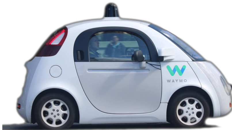
Figure 3.4: Autonomous cars depend on LIDAR sensors for perception. Here such a sensor can be seen on top of an autonomous vehicle prototype by Google's spin-off Waymo [194]. Adapted from Grendelkhan [56].
