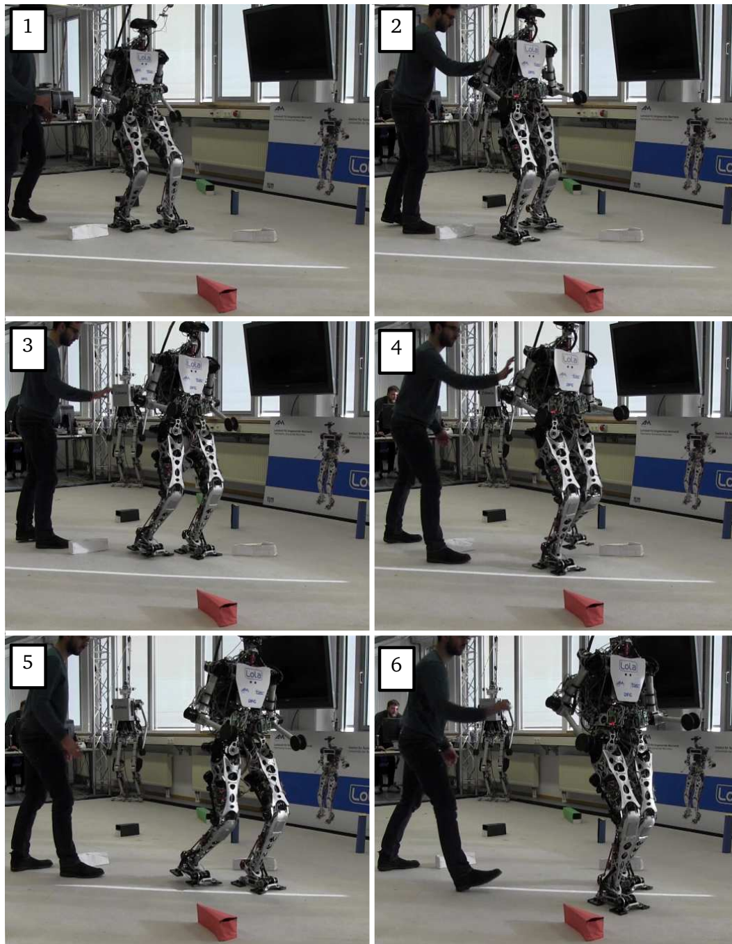
Figure 8.7: External Disturbances. From 1 to 6, the robot finds his way through cluttered terrain while being repeatedly disturbed by a human.
