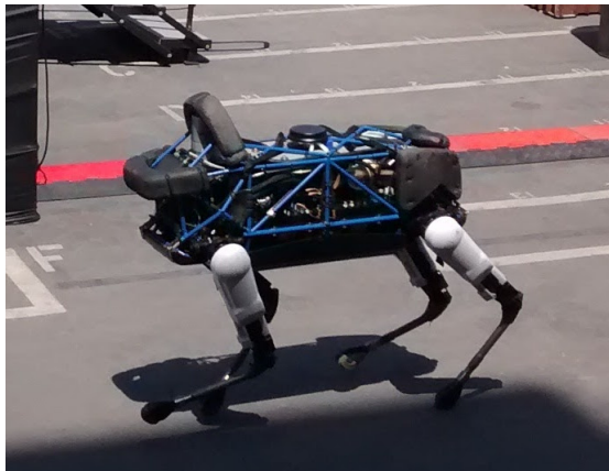
Figure 1.3: Legged robots with hydraulic actuation by Boston Dynamics. On the left, one of their latest quadrupeds, the 0.94 m-tall Spot (photograph by the author). On the right, the 1.8 m-tall Atlas humanoid robot, built for the DRC.
