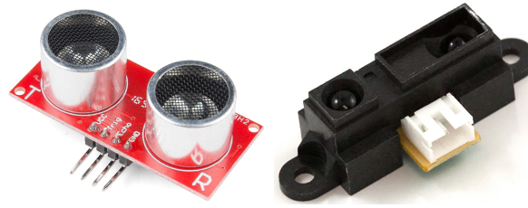
Figure 3.1: Unidirectional sensors are usually applied for proximity detection. Among the most popular types are ultrasonic (left) or infrared (right) [170].
