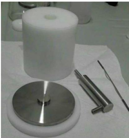
**Figure 2-10:** Tool used for the determination of the electric conductivity
