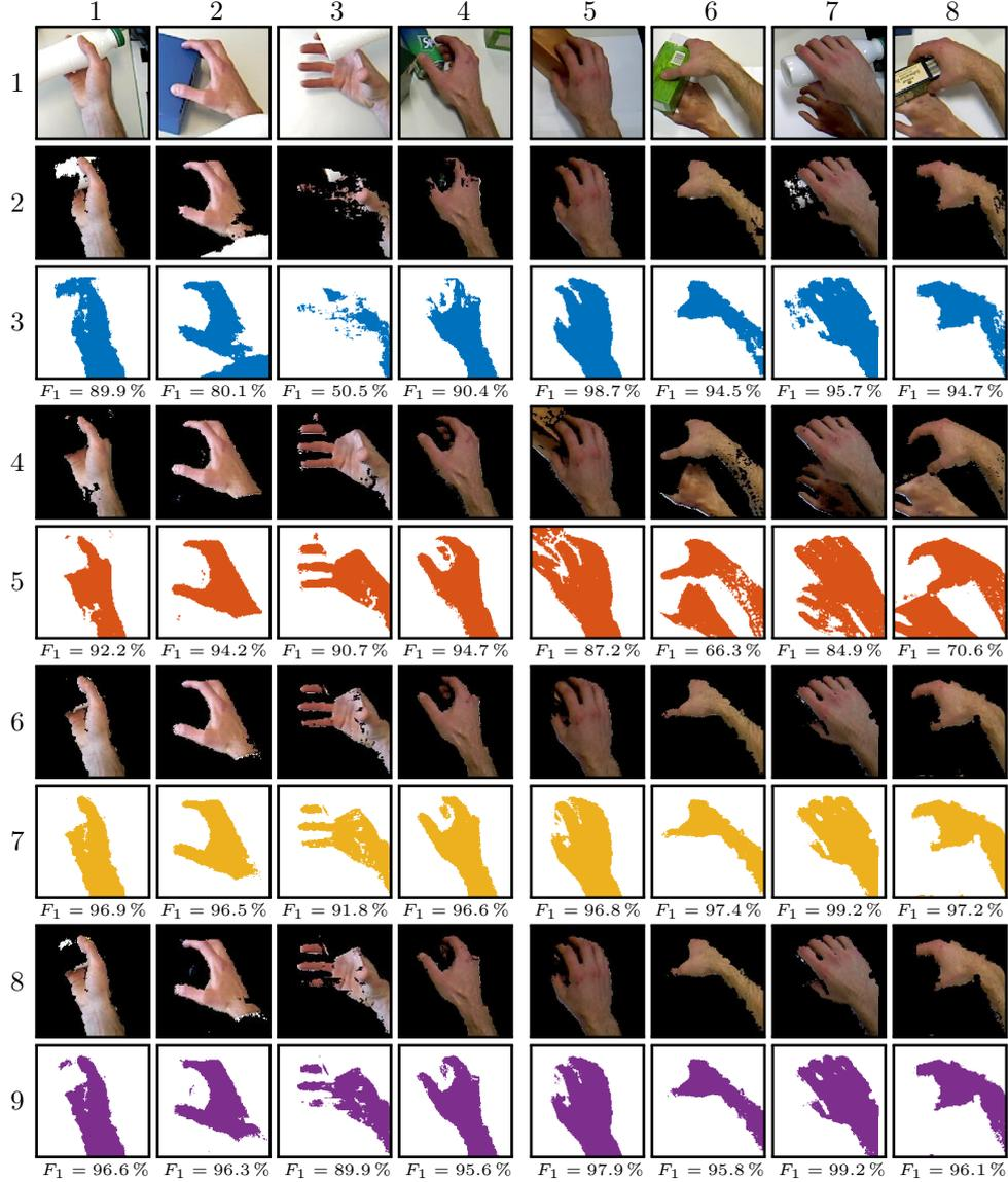
Figure 4.7: The figure shows segmentation results of the data sets EC1 (rows one to four) and EC2 (rows five to eight) containing extreme cases. An extreme case is defined as a situation where either  $f_{\text{RoI}}^{\text{depth}}$  excels  $f_{\text{RoI}}^{\text{color}}$  or vice versa. In general the structure of the figure is equal to Fig. 4.4, 4.5 and 4.6.
