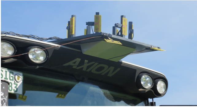
Figure 5. Uniform circular array prototype with 7 dipole elements, mounted on mowing machines roof. Two additional antennas for RFID-reader communication and received signal strength measurement.
