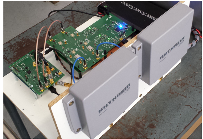
Figure 6. Prototype of hand-held receiver with 2 channel receiver and patch antenna array.
