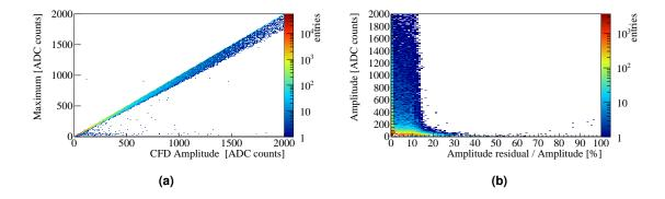
**Figure 3.7** Maximum value of one pulse as a function of the amplitude determined at the CFD sampling point (a). It can be seen that the amplitude determined with the second approach is in the range of 84 % to 100 % of the maximum. In (b) a similar picture can be seen, here the amplitude is plotted as a function of the relative distance to the maximum. Again a maximum deviation of 16 % can be seen. For small amplitudes the deviation is larger.
