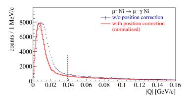
**Figure 5.25** Simulated data for  $\mu$ -Ni  $\rightarrow$  Ni $\mu$ - $\gamma$  reconstructed without the position dependent position correction applied (red) and with the correction active(blue). Enabling the correction leads to a much sharper peak structure.
