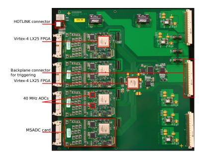
**Figure 3.1** Carrier-card with four mezzanine cards, important components are marked in the picture. The module is interfaced to the detecor by the four broad connectors on the left.
