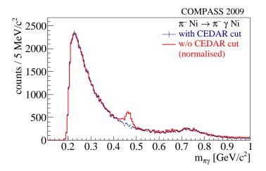
**Figure 4.14** Invariant mass distribution 2009, the selection without CEDAR cut is shown in red, the selection with CEDAR cut in blue. The histograms are normalized to the integral over masses smaller than  $0.4 \text{ GeV}/c^2$ .
