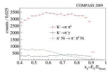
**Figure 4.19** Plot form which the  $\pi^0$ -background is extracted, yields as a function of  $x_{\gamma}$  are shown. The number of kaons decaying in the selected volume and which are detected in the final-state  $\pi^-\pi^0$ (red) the events where one photon is missed are shown in blue. In green the number of  $\pi^0$ s produced in the target are shown, this quantity is used for normalization.
