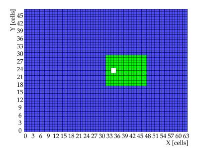
**Figure 3.4** Veto region for the single cluster trigger. Events are not triggered if the sum in the blue region is bigger than a given threshold plus the energy of the found cluster.
