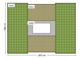
**Figure 2.9** The structure of ECAL1 [44] with the different cell types indicated. The beam hole is shown as white square.
