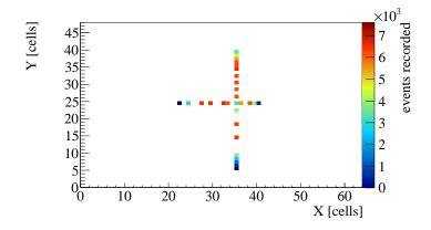
**Figure 3.15** Scan of the mapping of the ECAL trigger. An electron-beam is focused on one cell of ECAL2 and only this cell is activated in the trigger. Enabling only this cell in the trigger is used for verifying the mapping by showing the pattern of the detector movement. The variation in intensity is due to a different movement speed of the detector.
