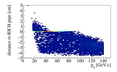
**Figure 2.12** Minimum distance of the scattered  $\pi^-$  from the RICH pipe as function of the pion momentum. A negative value indicates that the track fully lies within the gas-volume of the RICH pipe, while a value of zero indicates that the track crosses the RICH pipe. Only about 25% of the tracks travel a distance outside of the RICH pipe and thus may get a useful RICH information.
