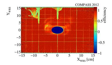
**Figure 5.37** Efficiency of the GEM detector GM05Y as a function of the position of the track in the wire reference-system (WRS). Negative values indicate points where no track was found or where the detector has its dead-zone. The grid structure is produced by the support elements of the detector while the broad patterns on top are produced by too much glue applied in these regions.
