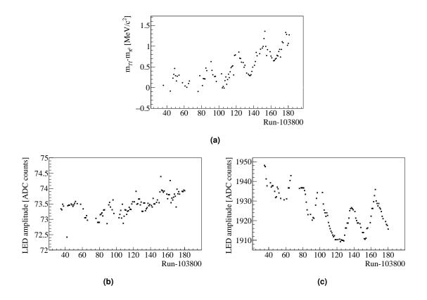
**Figure 5.13** Deviation of the  $\pi^0$  mass from the PDG value as function of the run number. The plot indicates the fluctuations within one week of data-taking. The fluctuations can be explained by thermal differences as expected from day-night changes.
