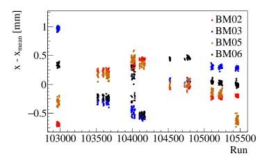
**Figure 2.2** Measured position of the BMS detectors as a function of the run number. The detectors BM01 and BM04 are not shown in this plot because they act as reference detectors for the alignment. This means their position is not a free parameter in the alignment procedure but the other planes are aligned relatively in a way that the precision of the reconstructed momentum is optimized.
