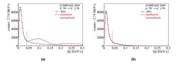
**Figure 4.6** (a) Distribution of the four-momentum transfer [1] in 2009 for pions. For better visualization the square-root of the distribution is taken. Slight deviations between the simulated events in red and the reconstructed data in blue stem from the structure of the calorimeter cells which is not reproduced in simulation. The cut is indicated as a dashed line. In (b) the same plot is shown for muon data.
