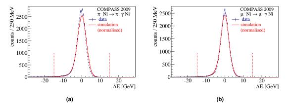
**Figure 4.7** Distribution of the energy balance[1] in 2009 for pions (a). Slight deviations between the simulated events in red and the reconstructed data in blue stem from the structure of the calorimeter cells which is not reproduced in simulation. The cut values are indicated as dashed lines. The same plot for muon data is shown in (b).
