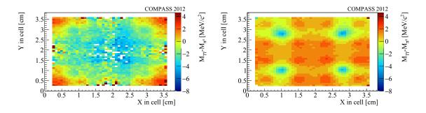
**Figure 5.22** Dependence of the reconstructed  $\pi^0$ -mass as a function of the reconstructed position inside a cell. In (a) a energy bin between 10 and 20 GeV is shown; in this case the mass tends to be reconstructed to higher values when the impact is close to the cell border. In (b) a energy bin between 60 and 70 GeV shows a more complex structure, around the four holding rods the mass is reconstructed at small values while around the light-guides it is reconstructed at higher masses.
