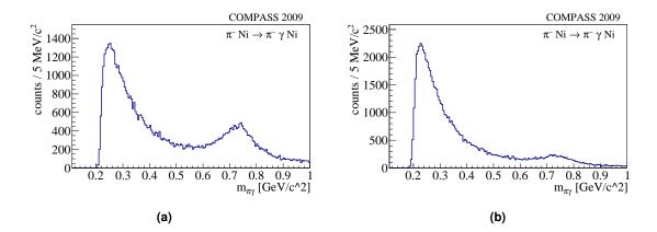
**Figure 4.10** Invariant mass distribution distribution of the  $\pi\gamma$  system. In (a) the cut on the number of photons in ECAL2 is not applied while it is applied in (b). A significant reduction of the  $\rho(770)$  contribution can be seen. Be aware that the selection in (a) was not performed with the final selection criteria.
