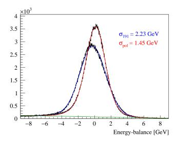
**Figure 5.11** Energy-balance distribution for the 3- $\pi$  final state. The histograms show the total energy of the final-state with a value of 191 GeV subtracted (blue) and the result of the polynomial parametrization subtracted (red). Both histograms are fitted with a sum of two Gaussians plus an arctan-function describing the background. The values extracted as  $\sigma$  are the RMS-widths when setting the background term, shown in green, to zero.
