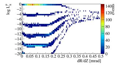
**Figure 5.9** Likelihood for tagging a pion as a proton in the 2012 data using a positive hadron beam with the CEDAR set up to detect protons. The likelihood gets split up into clean band corresponding to different multiplicities.
