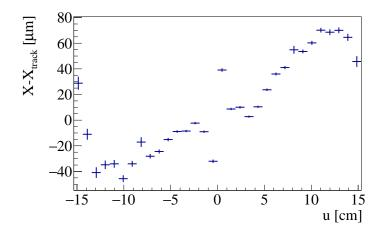
**Figure 5.28** Residual of GM01X as a function of the measurement point in the direction of measurement u. A linear slope in this quantity indicates alignment problems.
