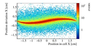
**Figure 5.24** Position deviation from the true position of a calorimeter cluster in X-direction as a function of the true position extracted from Monte Carlo data.
