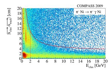
**Figure 4.3** Distance of the track, extrapolated to ECAL2, to the cluster position versus the cluster energy for all clusters. All tracks with momenta above 76 GeV/c are considered. The distance of correlated tracks depends on the cluster energy, the cut is indicated as a red line. The vertical, dashed line indicated the threshold below the clusters are not considered at all.
