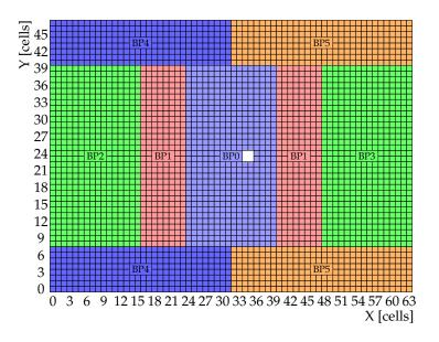
**Figure 3.9** Map of how the backplane modules are connected to ECAL2. BP0 is the most central module on which the trigger decision is taken.
