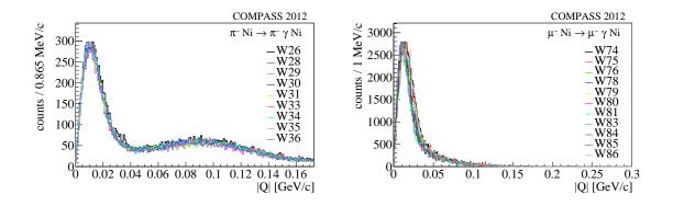
**Figure 5.31** Four-momentum transfer distribution measured in 2012 for  $x_{\gamma} > 0.4$ . The different measurement periods are indicated by colors. All histograms are normalized to the maximum. The left panel shows pion data and the right panel muon data.
