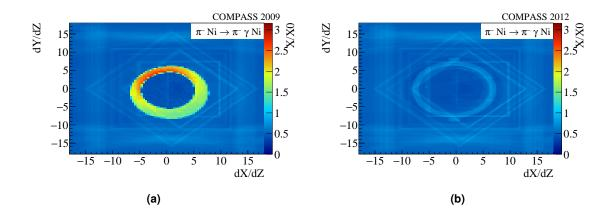
**Figure 2.11** Distribution of the material budget expressed in radiation lengths seen by a neutral particle extrapolated from the target to the surface of ECAL2 as a function of the angle relative to the z-axis. The setup from 2009 (a) shows a prominent circular enhancement corresponding to the steel RICH-pipe. In the setup used in 2012 (b) this enhancement is significantly reduced.
