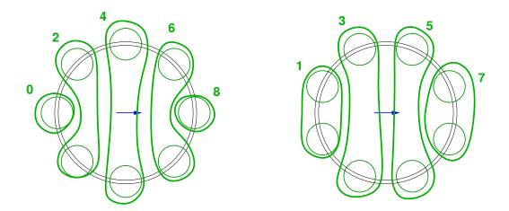
**Figure 5.3** Mapping of the CEDAR PMTs in different groups G0,G1,...,G7 as used in the text, as a function of the beam direction [85]. The blue arrow indicates the beam direction and the PMTs are shown as circles which are combined into groups of one or two PMTs depending on their position.
