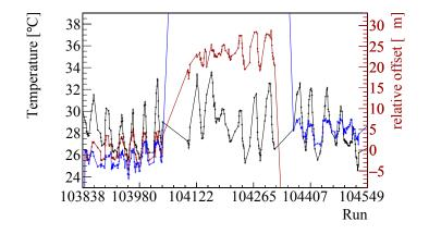
**Figure 5.27** The measured temperature in the COMPASS hall as a function of the run number shown in black. Superimposed in red the relative movement of "SI01U" (red) and "SI01V" (blue). It can be seen that the position follows the day-night fluctuations of the temperature while at the edge between two periods the position jumps by an arbitrary number.
