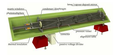
**Figure 2.10** Cross section through one CEDAR detector. For more details about the various components c.f. [44].
