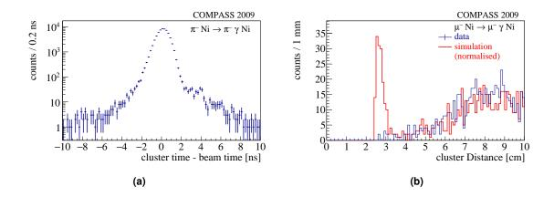
**Figure 4.2** In (a) the time distribution relative to the beam time for all clusters matching the selection criteria for the reaction  $\pi^-\text{Ni} \rightarrow \text{Ni}\pi^-\gamma$  is shown. Only clusters in a time-window of  $\pm 8$  ns are used. In (b) the radial distance between all reconstructed clusters is shown for data in blue and for the simulation in red. It can be seen that an artificial peak at cluster distances around 3 cm is created in simulation.
