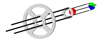
**Figure 2.4** The target used for 2012 data-taking as it is implemented in Monte Carlo. The support structures consisting of stainless-steel are shown in grey, the carbon holding-rods are shown in black. The 4 mm nickel-target is indicated in red. The 25  $\mu$ m tungsten target is shown in blue and the 50  $\mu$ m one in green.
