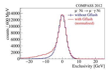
**Figure 5.34** Exclusivity distribution obtained from the 2012 data compared with the TGEANT simulation. In case the "Gflash" parametrization is used (a) the simulated width is too high. In case the full shower simulation is applied (b) the spectra mathc nicely.
