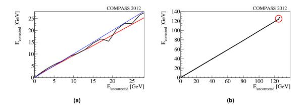
**Figure 5.21** Misbehaving energy dependent calibration coefficients. In (a), bin by bin fluctuations are seen while in(b) problems with the end-point of the fit become visible.
