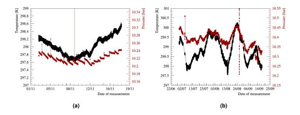
**Figure 5.8** Temperature (black) and Pressure variations(red) in CEDAR 1. In (a) the pressure was manually adjusted leading to a step-like structure. In 2012 (b) this adjustment was performed automatically and the structure is more smooth.
