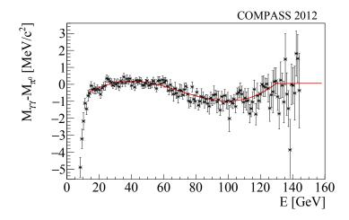
**Figure 5.20** Fitted energy dependence of the  $\pi^0$ -mass using an interpolating function. Binby-bin fluctuations are removed by this function. In region with a strong energy dependence the function is not used.
