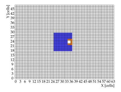
**Figure 3.2** Map of selected cells for the summation trigger. The cells depicted in blue are chosen while the cells shown in orange are excluded in order to be less sensitive to elastically scattered beam-particles.
