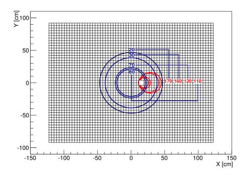
**Figure 3.5** Distribution of the positions the final-state particle hits ECAL2 as a function of energy [63]. The photons are shown in blue and the pions in red.
