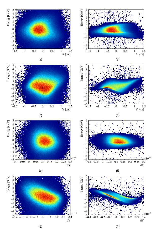
**Figure 5.12** Dependence of the beam-energy on the spatial beam-parameters. On the left panels the energy is determined from the  $\pi^{-}\pi^{-}\pi^{+}$  final-state. On the right the beam-energy is given by the polynomial parametrization of the beam.
