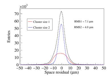
**Figure 2.5** Spacial residual of one exemplary silicon plane [44]. The residual for hits spanning one detector strip and hits is shown individually as well as the integral which is shown in black.
