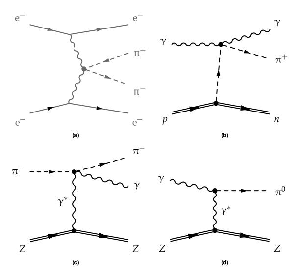
**Figure 1.3** (a-c) show processes embedding the pion Compton scattering. In (d) the original Primakoff process is shown.
