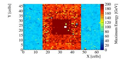
**Figure 2.8** Maximum measurable energy per cell in ECAL2. The different regions are adopted to the different maximum photon energies which are expected.
