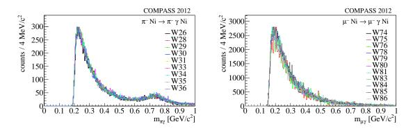
**Figure 5.30** Invariant mass distribution of the  $\pi\gamma$ -system measured in 2012 for  $x_{\gamma} > 0.4$ . The different measurement periods are indicated by colors. All histograms are normalized to the maximum. The left panel shows pion data and the right panel muon data.
