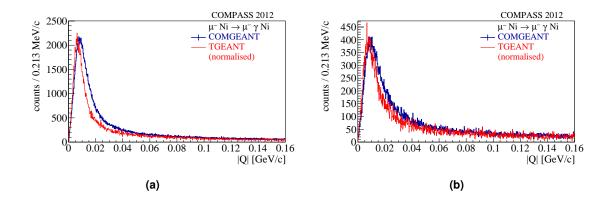
**Figure 5.36** Difference between the reconstructed four-momentum transfer distribution for events generated by COMGEANT (blue) and TGEANT (red). The spectra in (a) agree less than in (b) where a cut on the residual of the primary vertex is performed.
