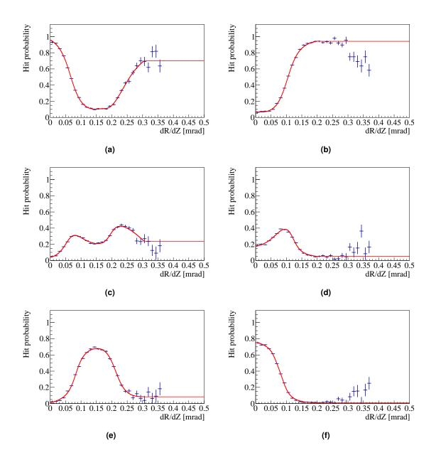
**Figure 5.5** Hit probability for the PMT group G1 for pions (left) and kaons (right) as a function of the beam inclination. From top to bottom the probability for no hit, one hit and two hits is shown. The red line indicates the parametrization obtained by a fit.
