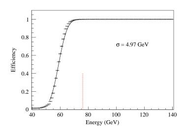
**Figure 4.1** Efficiency of the ECAL2 trigger in 2009. The Distribution is fitted with an integrated Gaussian. The red dashed line corresponds to the applied threshold of  $E_{\gamma} = 76 \text{ GeV}$  used in the analysis. The value quoted as sigma is the width of this fit[44].
