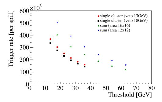
**Figure 3.18** Threshold scan for the Primakoff triggers. The individual trigger rates a shown as a function of the threshold. For the summation triggers two different areas are scanned. For the single cluster trigger also the veto threshold is changed.
