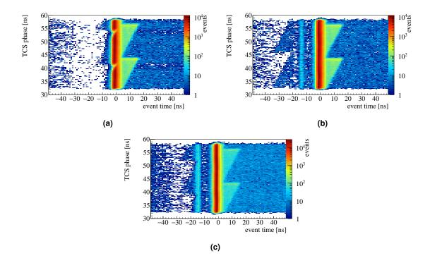
**Figure 3.16** Trigger time as a function of the TCS phase for different trigger time gates. The events where the calorimeter-trigger matches the beam-trigger are indicated by a vertical, red band while the triangular shapes indicate pile-up. A gate of 26 ns is too narrow and part of the interesting events are cut away (a). A gate of 48 ns is to big and allows for too much pile-up (b). A time gate of 42 ns is chosen to allow a relatively low amount of pile-up (c).
