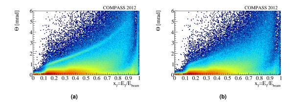
**Figure 4.17** Scattering angle vs. the momentum of the scattered muon. In order to have a larger kinematic range, it is visualized from 2012 data. The picture is shown with no cuts applied (a) where an enhancement is seen at large scattering angles forming a band along the upper limit. This band is created by  $\mu^-e^-$ -scattering. Cutting on the number of additional tracks in the spectrometer (b) significantly reduces this background where contributions only remain at high muon momenta.
