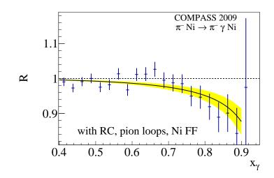
**Figure 4.25** Ratio plot between data and simulation including radiative corrections, chiral loops and the contribution from the Nickel form-factor. The yellow band indicates the error on the fitted curve from which the polarizability value  $\alpha_{\pi} = (2.0 \pm 0.6_{\text{stat.}} \pm 0.7_{\text{syst.}}) \times 10^{-4} \text{ fm}^3$  is extracted.
