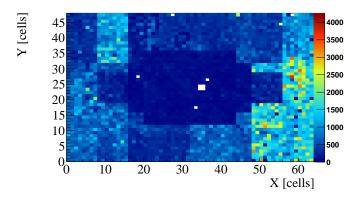
**Figure 2.7** Distribution of LED amplitudes per cell for ECAL2. It can be seen that the inner part consisting of Shashlik cells has only little response on the LED amplitude. Additional rectangular structures in this plot stem from different LEDs used for different regions.
