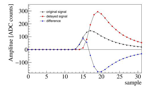
**Figure 3.6** Illustration of the implementation of the CFD algorithm. The signal coming from the detector(black triangles) is delayed by two clock cycles and amplified by a factor two (red circles). The difference between these two signals shown as blue squares is used to detect the signal.
