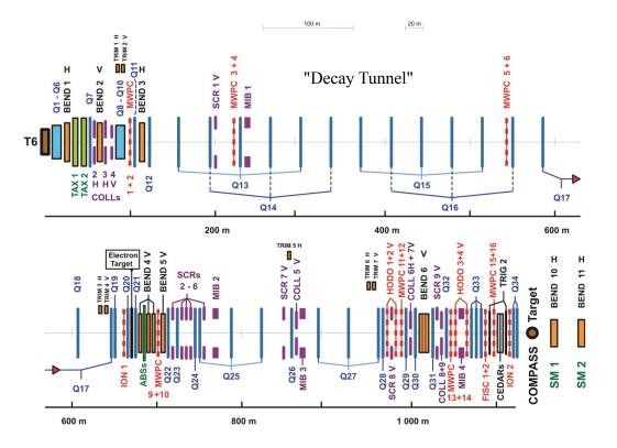
**Figure 2.1** Sketch of the M2 beam-line. The focusing quadrupole magnets are indicated with "Q" while the dipole magnets are indicated by "BEND". In order to absorb electrons from the hadron beam the "Electron target" is installed. In case of muon beams the "ABSs"<sup>*a*</sup> is installed absorbing remaining hadrons from the beam.
