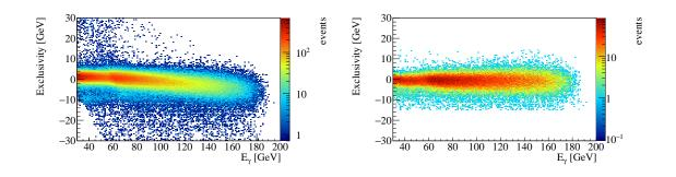
**Figure 5.23** Energy dependence of the exclusivity before correction (a) and after the position dependent energy correction is applied (b).
