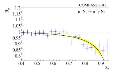
**Figure 5.35**  $x_{\gamma}$  ratio for part of the muon data taken in 2012 with the current TGEANT simulation. A false polarizability of  $\alpha_{\mu}^{\text{false}} = 2.5 \times 10^{-4} \text{ fm}^3$  is extracted.
