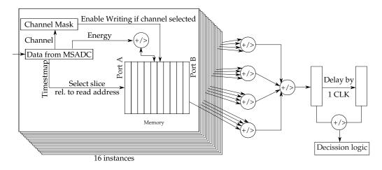
Figure 3.12 Data flow for the processing on the backplane card.
