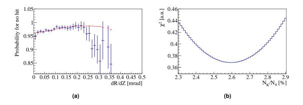
**Figure 5.10** Distribution for no-hit probability in PMT group G6, c.f. fig. 5.3, (a) in case of the pion sample (blue). In red the distribution as it would be expected from a ration  $N_K/N_\pi \approx 2.6\%$  is shown. In (b) the  $\chi^2$  distribution when minimizing the difference between the two histograms in (a) is shown.
