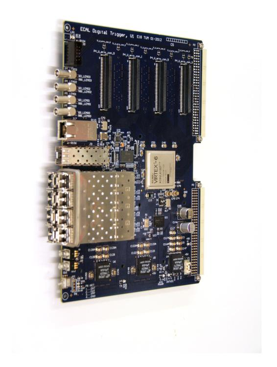
**Figure 3.10** The backplane card used in 2009. On top the connectors to the carrier-cards are shown. On the left top the LEMO outputs providing the trigger signals are placed. Below the not used Ethernet connector is placed above the TCS receiver. On the bottom the 2x4 SFP cage provides the high-speed serial links. All data are processed by the Viretx-6 FPGA in the center.
