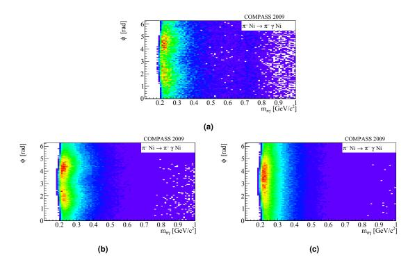
**Figure 4.13**  $\phi$ -angle between production and decay plane as a function of invariant mass. It can be seen that the distribution from measured data (a) agrees with the simulation based on the [78] generator(b) while the Polaris generator (c) shows a different distribution.
