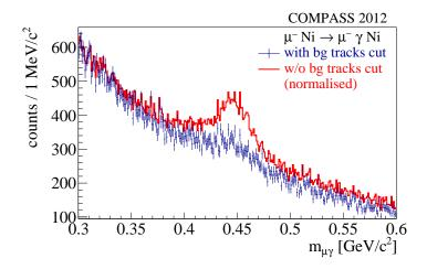
**Figure 4.16** Invariant mass of the  $\mu^-\gamma$  system, zoomed around the calculated mass for muonelectron scattering. The blue curve shows the effect of the cut on the number of background tracks compared to the red curve where this cut is not applied.
