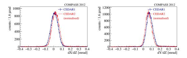
**Figure 5.1** CEDAR tilt-direction:  $dX/dZ_{CE}$  left panel,  $dY/dZ_{CE}$  right panel. CE01 is shown in blue CE02 in red.
