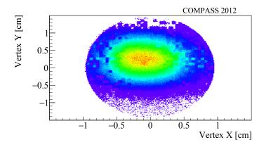
**Figure 5.4** Vertex distribution with a binned CEDAR calibration, bin-by-bin fluctuations in the efficiency are visible as speckles in the *XY* distribution of the vertex. Data with radii bigger than 1 cm are excluded as no reasonable calibration is expected due to limited statistics.
