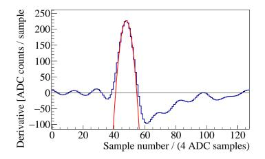
**Figure 5.16** Example of the derivative of the pulse extracted with the FFT based algorithm on ECAL2. The blue line shows the derivative with an increased number of "samples" by a factor of four. The red line indicates the parabola with which the shape is approximated.
