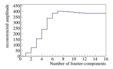
**Figure 5.18** Reconstructed amplitude as function of the number of fourier components used. The plot has been extracted for one exemplary pule with an amplitude of 415 ADCcounts. The amplitude is maximum between seven and eight components.
