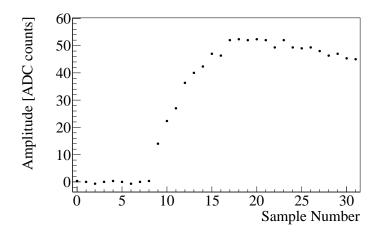
**Figure 5.14** Example of a noise pulse. Here a discharged cell slowly recovers up to the nominal baseline value of 50 ADCcounts.
