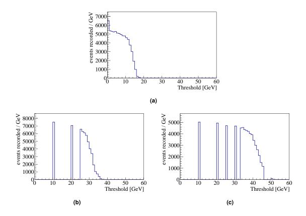
**Figure 3.14** Threshold scan of the ECAL-trigger with an electron beam of three different energies: 15 GeV (a), 30 GeV (b) and 40 GeV (c). For each threshold the number of triggered events in one spill is shown which decreases as soon as the threshold exceeds the average beam energy. In case the plots indicate zero events the measurement was not performed at that threshold.
