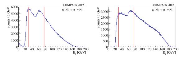
**Figure 5.29** Distribution of photon energies measured in 2012 applying the same cuts as for the 2009 data. The dip in the distribution stems from the two different triggers, where the trigger with a lower threshold is scaled by a factor of two. The vertical lines indicate the range which may be used for analysis and for which the number of events is extracted. The left panel shows pion data and the right panel muon data.
