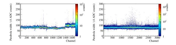
**Figure 5.17** Width of the parabola assumption for the derivative of the FFT based amplitude as a function of the channel number. In (a) the distribution is shown for ECAL1 and a strong dependence on the cell type is visible. In (b) the distribution is shown for ECAL2 here a more unform distribution is extracted.
