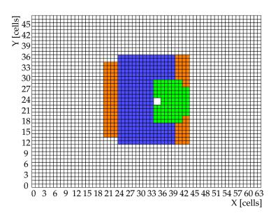
**Figure 3.3** Map of selected cells for the maximum cluster trigger. The cells depicted in blue are chosen while the cells shown in orange are used as one combined cell in case the maximum cluster is close to those regions. The cells shown in white and green are not included into the trigger
