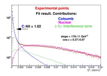
**Figure 4.21** Fit to the  $Q^2$ -spectrum over the total  $x_{\gamma}$ -range[89]. The data is fitted with a component stemming from strong interaction given by eq. 4.6 (magenta) smeared with the experimental resolutions, a component from the Primakoff process extracted from simulation (blue) and an interference term (green).
