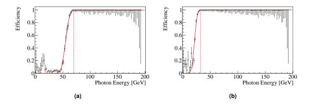
**Figure 3.21** Efficiency of the Primakoff triggers as function of the energy of the cluster with the highest energy inside the trigger region. A fit with an integrated Gaussian gives a width for the rising edge of P1 of  $\sigma$ =5.7 GeV (a) the efficiency plateau of 99% is reached at 70 GeV in this case and is indicated as dashed line. P2 has a slightly smaller width of  $\sigma$ =3.9 GeV and reaches its plateau at 32 GeV.
