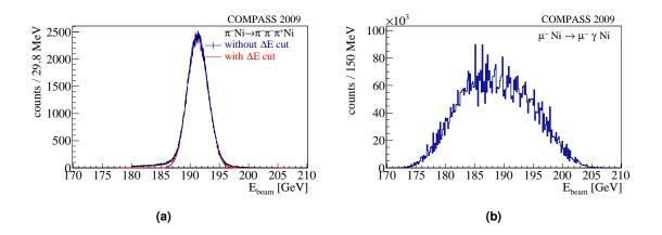
**Figure 4.11** Distribution of the beam energy in 2009 for a pion beam (a) and a muon beam (b). In (a) the distribution of all  $3\pi$ -events is shown in blue and with the cut on the beam energy given by the parametrization is shown in red. In (b) the distribution measured by the BMS is shown.
