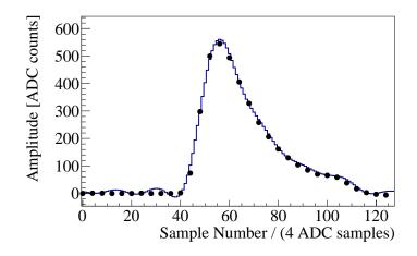
**Figure 5.15** Example pulse from ECAL2. The measured data points are shown as black dots. The pulse shape reconstructed from eight fourier-components is shown as blue line. The fourier transformation allows to effectively consider the pulse as if it has more samples. In this case the number of samples is visualized with a reduced spacing by a factor of four.
