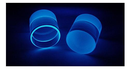
Figure 2.6: Two scintillating  $CaWO_4$  crystal irradiated with UV light. The scintillation light is in the blue range of the visible spectrum. The front face of the right crystal is roughened which visibly homogenizes and enhances the light output.
