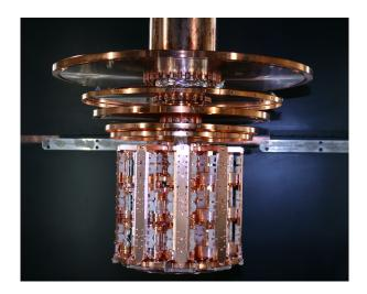
Figure 2.2: The carousel was designed to hold up to 33 detector modules (equivalent to a total target mass of 10 kg). In the upper part of the picture the flanges for connecting the thermal shields and the vacuum chamber are visible.
