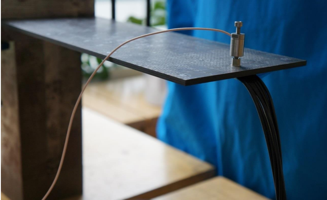
Figure 9.7 Experimental setup of vibration configuration on specimen 1
