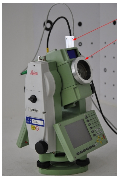
Figure 4.9 – Prototype of an Image Assisted Total Station (Reiterer and Wagner, 2012)
