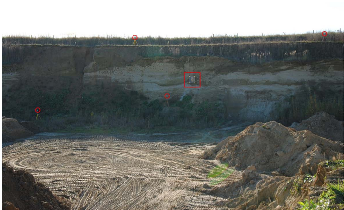
Figure 4.15 – Region of interest (ROI) with highlighted control points and artificial rock
