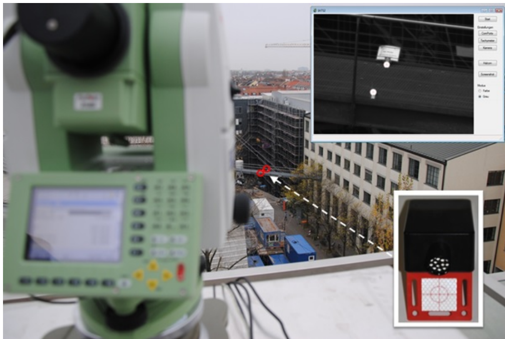
Figure 4.3 – Test measurement at TUM campus with screenshot (top right) and used LED target (bottom right)
