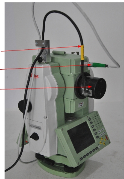
Figure 4.9 – Prototype of an Image Assisted Total Station (Reiterer and Wagner, 2012)
