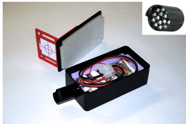
Figure 4.2 – LED target in self-made isolated housing. Detail of LED cluster top right
