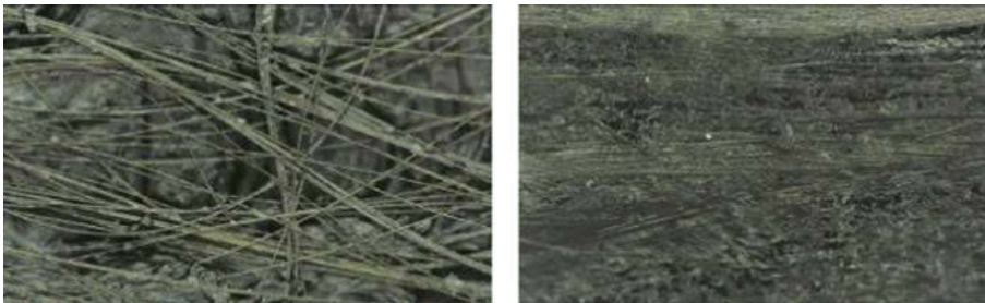
Plate 1. Rubber (SBR) pressed into fibers at 250-400bar at KRAIBURG Gummiwerke
