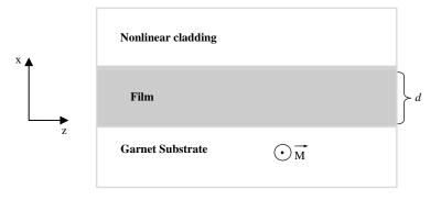
Figure 1. Basic geometry of the sensor
