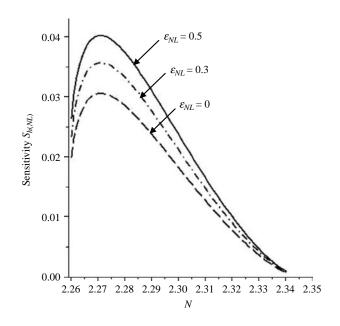
Figure 3. Sensitivity of the sensor with structure consisting of a nonlinear cladding, a linear film, and a MO substrate measured as function of the effective refractive index (N) at different values of  $\varepsilon_{NT}$
