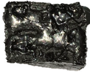
Fig. 4-58: Typical resin squeeze-out observed at the tip of a thermoplastic composite material specimen after testing [S10]
