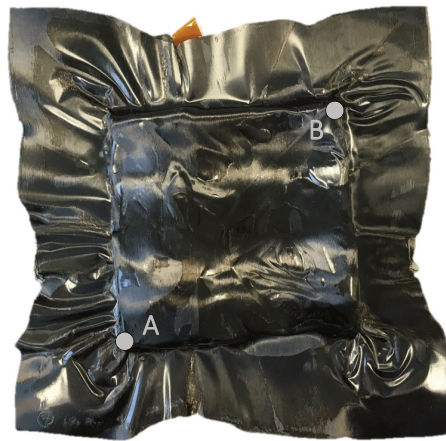
Fig. 6-6: Thermoforming outcome of the [0_2 90_2]_s tailored blank Points A and B are given for orientation purposes (see Fig. 6-1).
