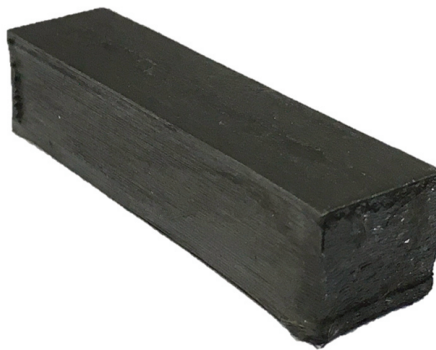
Fig. A-15: Prismatic bar specimen made out of non-cured unidirectional thermoset tapes
