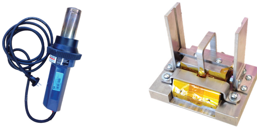
Fig. A-9: Heat gun used to heat thermoplastic specimens above melting temperature (left) and specimen preparation tooling protected with kapton tape (right) [S8]
