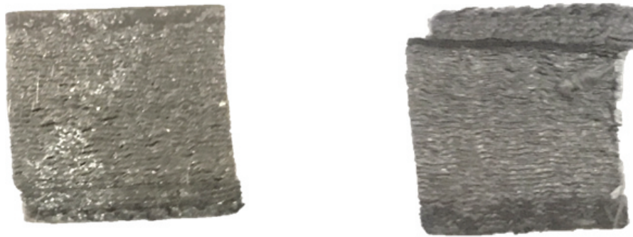
Fig. A-16: Typical (left) and extreme (right) localised inter-ply shear deformations at the tips of the specimen
