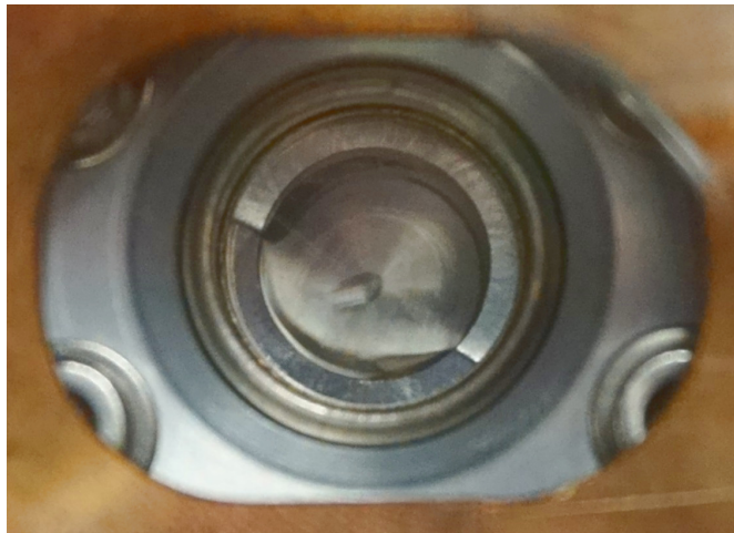
Figure 4.5.: Deuterium frozen in the irradiation cell. The crystal is transparent and can hardly be seen. The diameter of the inner cell volume is 12 mm.
