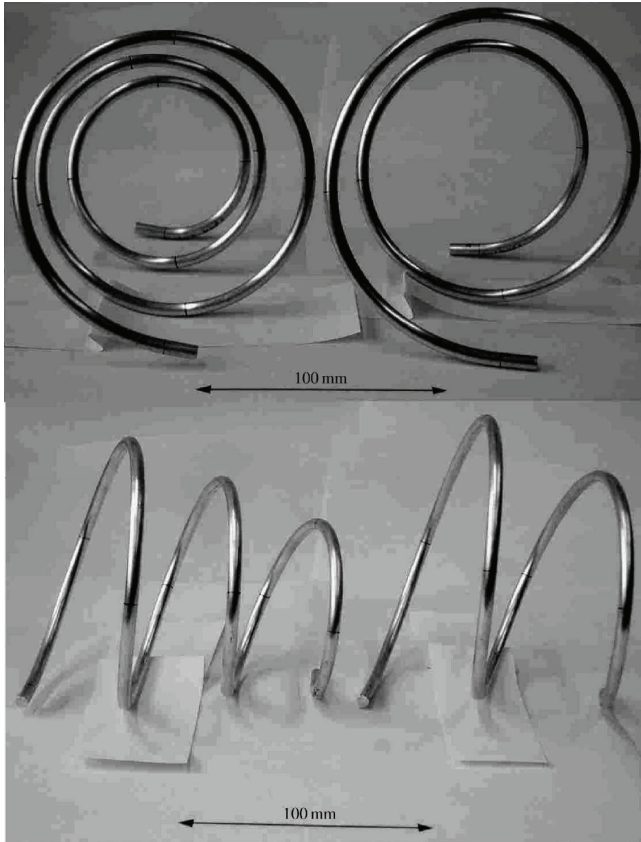
Fig. 5 Formed conical spirals with lengths a = 759.5 mm (right hand) and a = 954.4 mm (left hand)
