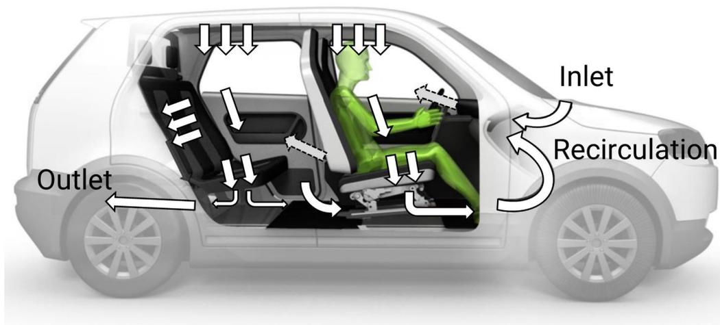
Figure 17: Vertical air flow distribution in prototype vehicle EVA (Stuke & Bengler, 2013)
