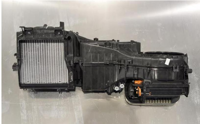
Figure 18: HVAC unit, takeover part from a VW Jetta
