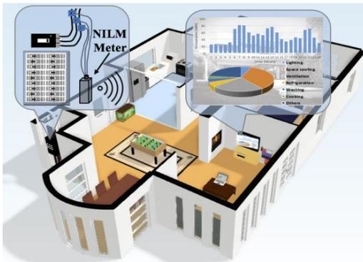
Fig. 1: Non-Intrusive Load Monitoring (NILM)
