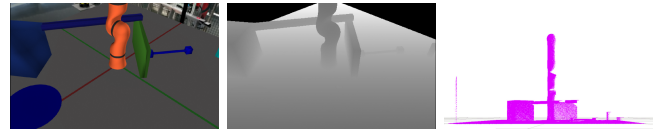
Fig. 5. RGB image (left) and 2.5D depth stream (middle) sent by the sensor, and the resulting 3D PC (right).
