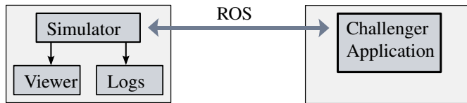
Fig. 2. Platform provided by challenge 2 host including the (Gazebo-based) simulator, the ROS simulator-interface and the challenger application.
