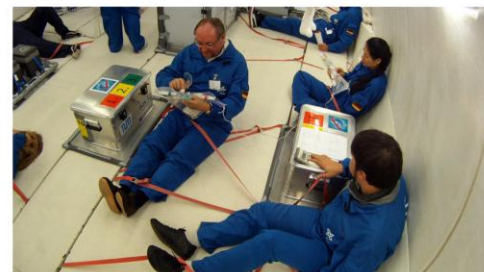
Fig. 4 Conducting the experiment on early ettringite crystallization onboard the zero g airplane. Note that all experimenters are fixed to avoid free floating during the zero gravity period.
