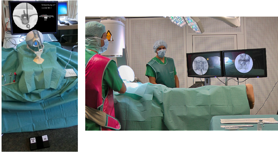
Fig. 37: (Left) Our stand-alone VR simulator with C-arm control and haptic feedback. (Right) Our simulator in a controlled medical simulation setting at the Institut für Notfallmedizin und Medizinmanagement, Munich, Germany.
