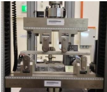
Figure 5-4: Four-point bending test setup
