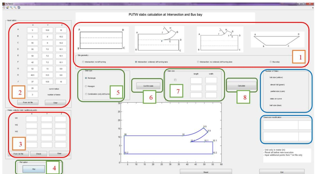
*Example:* Calculation of PUTW slabs for an intersection with widened left-turning lane (3 lanes, 10.8 m width, 52 m length) with boundary co-ordinates of construction site stored in text file; additional points are collected later then input manually. Details are showing as below table:
