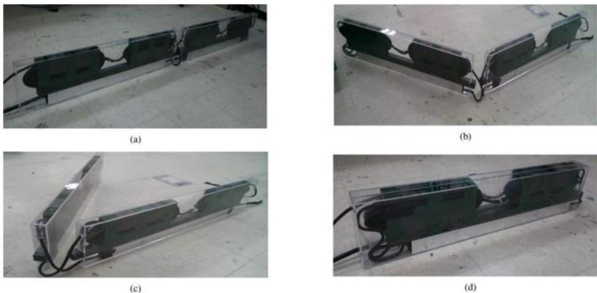
Figure 3-18: Foldable S-type power supply modules: (a) fully deployed case, (b) one-third folded case, (c) two-thirds folded case, (d) completely folded case (Choi, et al., 2015)
