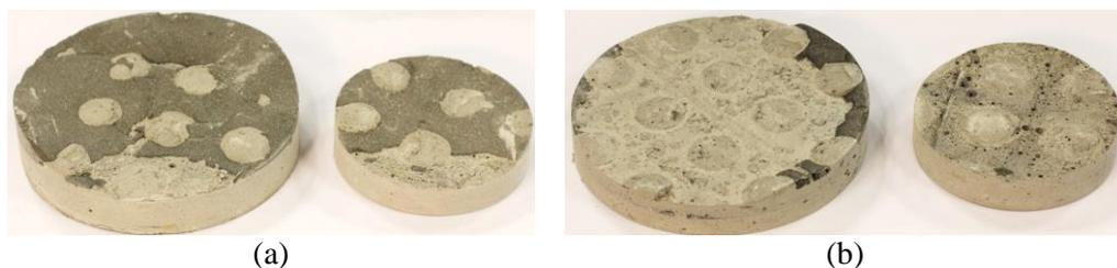
Figure 6-12: Failure types in sample with circular convex nodes in shear test
