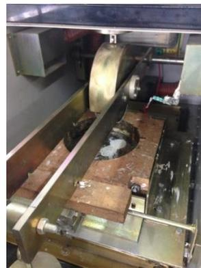
Figure 5-12: Wheel Tracking Machine
