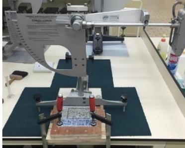
Figure 5-10: British Pendulum Tester (BPT)
