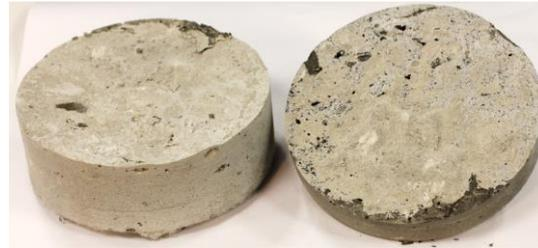
Figure 6-14: special failure type of sample with flat contact in shear test
