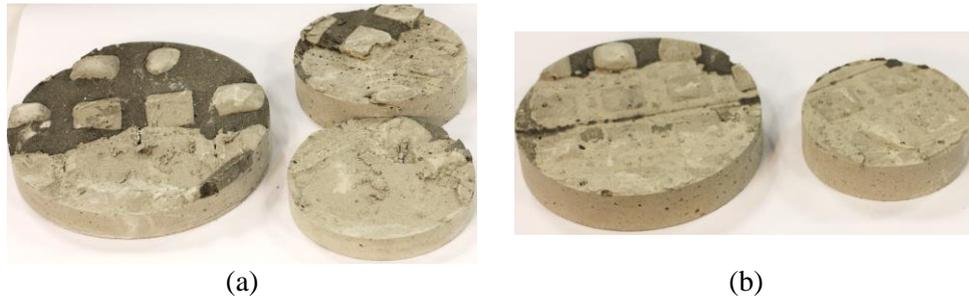
Figure 6-13: Failure types in sample with square convex nodes in shear test
