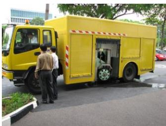
Figure 2-2: Sideway-force coefficient routine investigation machine (SCRIM) (LTA, 2012)
