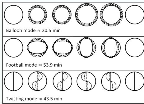
dal free oscillations. Toroidal free oscillations cause variations only in horizontal direction whereas spheroidal free oscillations cause variations in vertical and horizontal directions. In contrast to the pendulum, a gravimeter measures only spheroidal oscillations, because gravimeters can measure only the vertical motions. The three ground modes of free oscillations are shown in Figure 2.3.4.
