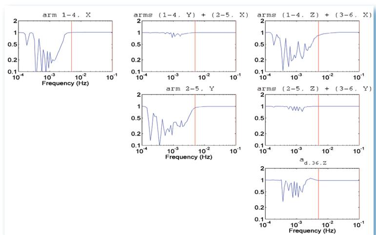
Fig. 1.3.2: Ratio between the errors of the differential acceleration after and before external calibration. Results are based on simulated GOCE data.
