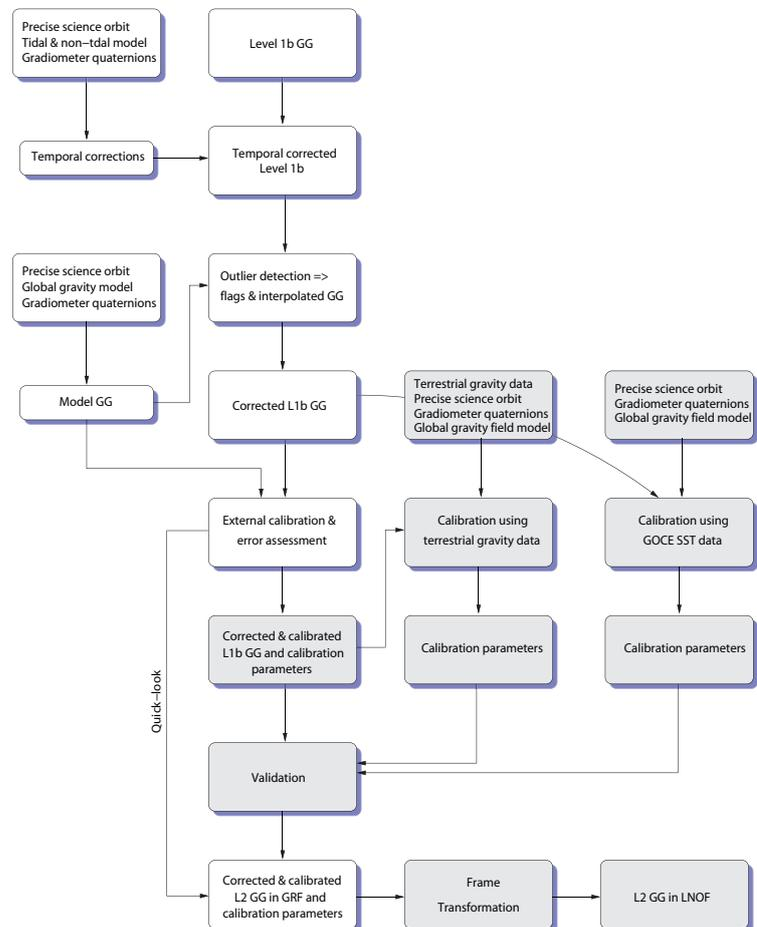
Fig. 1.3.1: Flowchart of gravity gradient preprocessing at the GOCE HPF. The blocks in grey are part of the final mode only.
