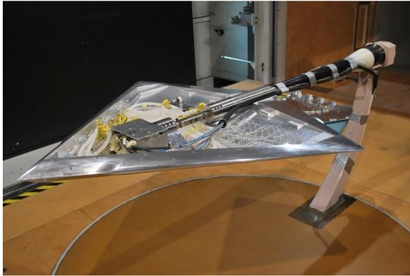
Figure 3.8: SAGITTA W/T model without the pressure side shell.
