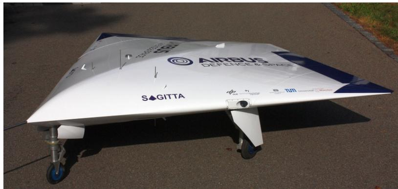
Figure 1.8: SAGITTA demonstrator configuration.
