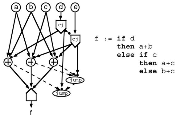
Fig. 4: A CDFG with jumps inserted and the corresponding nested conditional expression.
