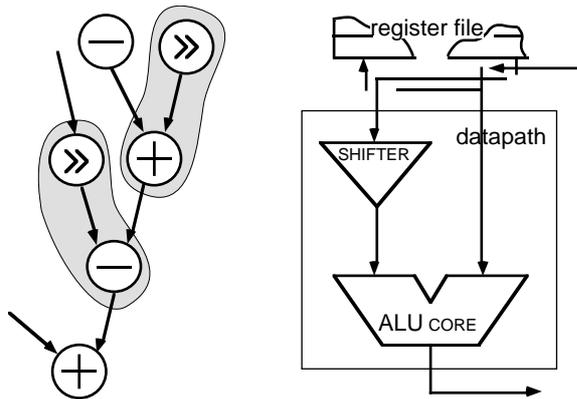
Fig. 5: A CDFG with possible clustering and a simplified datapath for which the clustering was constructed.
