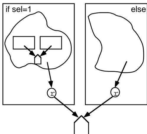
Fig. 3.b: The clusters are marked with the conditions. This transformation is applied recursively to the CDFG possibly resulting in nested conditions.
