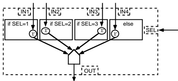
Fig. 2.c: Four different definitions of an operand are merged. The definitions are merely renamings. Each operand depends upon a condition which is the equality of the selector with the appropriate setting.
