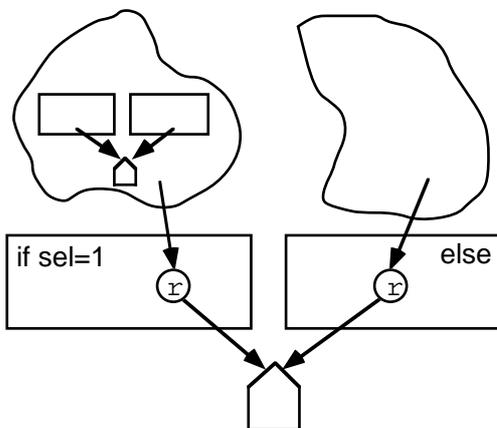
Fig. 3.a: Conditional operations and data-dependent clusters prior to the transformation
