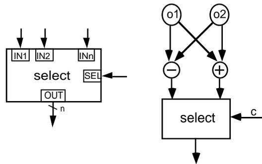
Fig. 2.a: The template for an n-way select operation.
