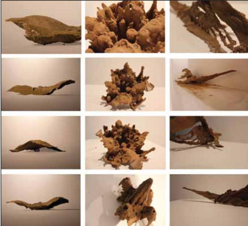
The research is structured. The outcome: the surface is a series of shells, columns and dome structures created by spraying, injecting and dripping various chemicals on sand. The shell structure can extend to a large span in the desert, creating below it large spaces covered in a surface made of sand. After creating the shell structure, I started applying the adhesive differently, by injecting. This helps in accumulating sand and lets it adhere to each other, creating columns.
