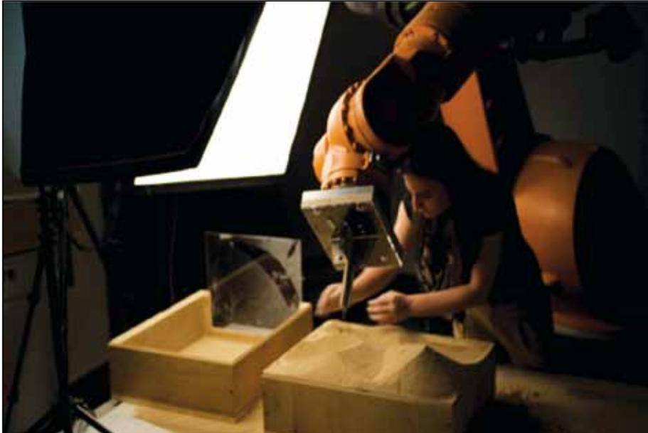
The research is structured around several prototypes built to investigate the potential methods of applying an adhesive to solidify the structure. The process reveals the stages of freezing the sand and turning it into building units by using robotic interventions.
