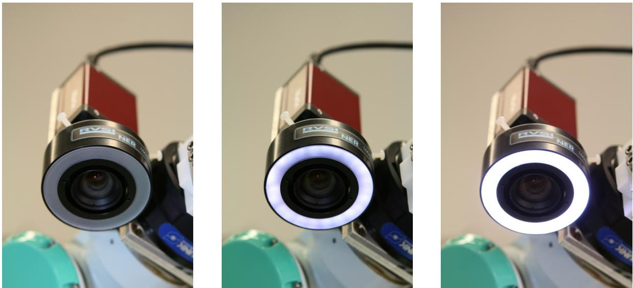
Figure 6. The light-source attached to the robot's tool in off-state, 30 % and 100 % brightness.
