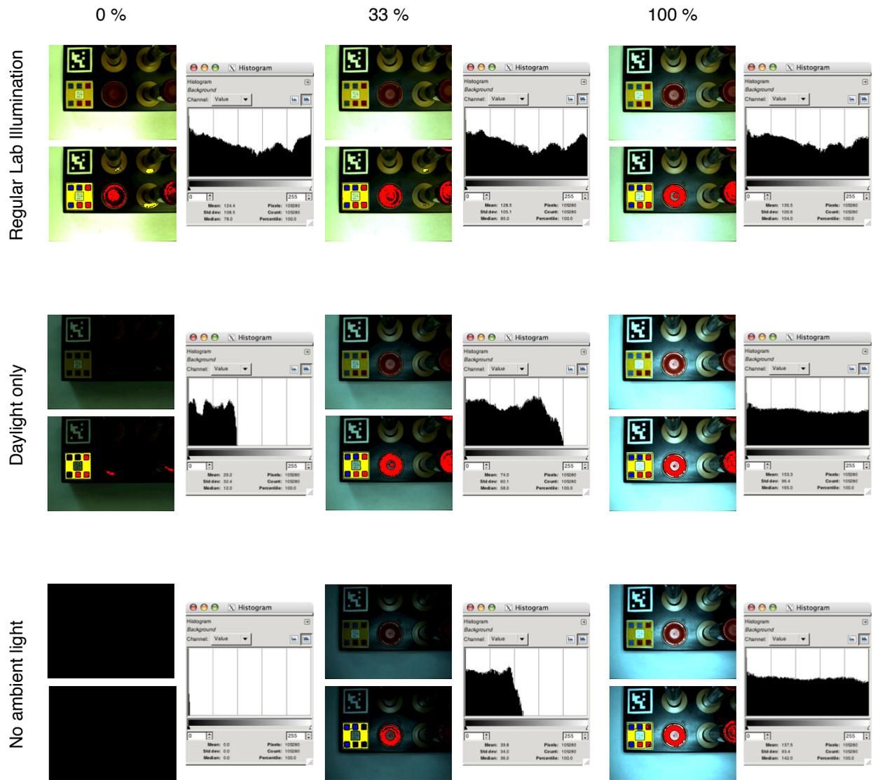
Figure 9. Color segmentation at the Vacutainer rack. The color segmentation shows constantly very good results if the ceiling lights in the lab are on. In the darker scenarios color segmentation works significantly better, with the additional illumination by the LED array.
