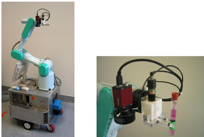
Figure 1. The mobile robot platform for automation of sample management processes. The close-up picture on the right shows the robot arm's tool with the red camera pointing down for object detection and the two fingered gripper for grasping vials of different sizes.
