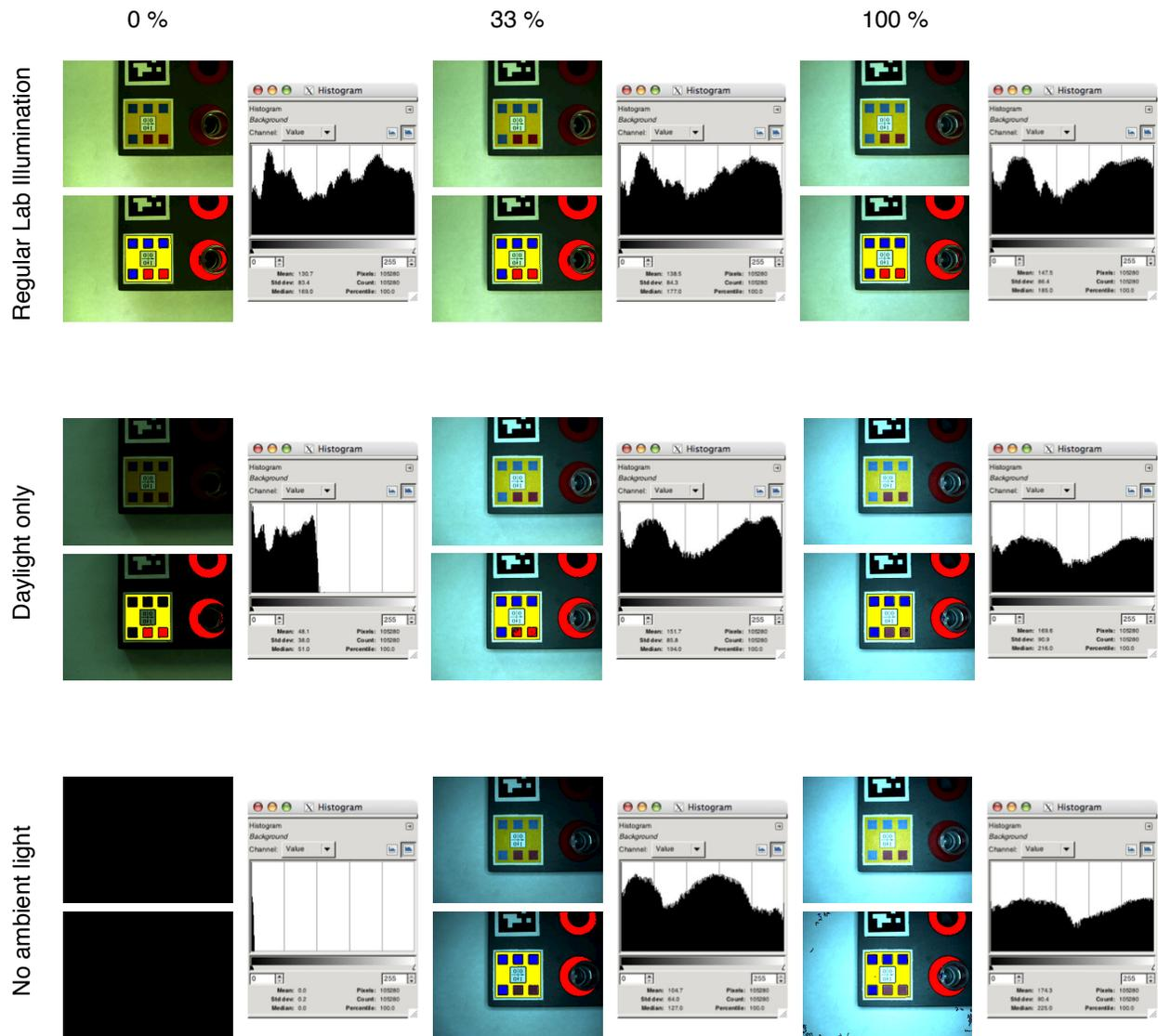
Figure 8. Color segmentation at the Cedex rack. While the color segmentation shows very good results in all cases when the ceiling lights are switched on in the lab, it becomes much harder to examine the colors in a lab when the ceiling lights are off, be it day or night. The LED array significantly improves color detection in the latter cases.
