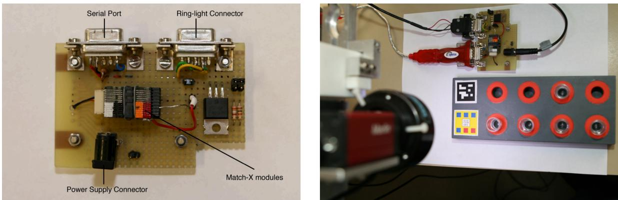
Figure 5. The controller board with the serial and the ring-light connector next to the Match-X stack consisting of two modules in this case. The right picture shows the mounted test setup for verifying the results.
