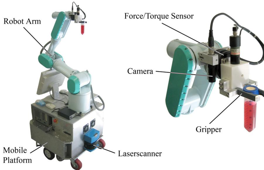
Figure 2. The mobile robot platform with its sensors and a close-up of its tool.
