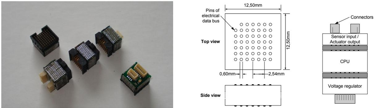
Figure 3. Some exemplary modules out of the Match-X construction kit are depicted on the left, while the center image shows the data bus layout. The right image shows an elementary assembly of three blocks with a CPU, a voltage regulator and sensor connectors.
