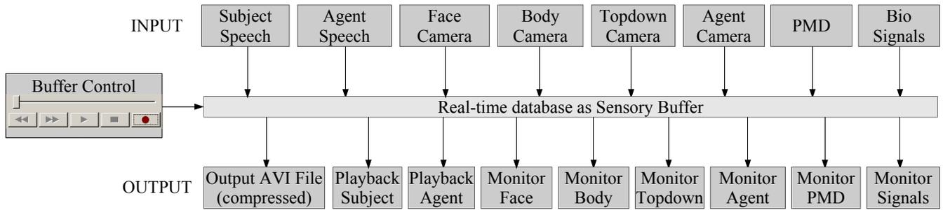
Fig. 1. Overview of the multi-modal recording scheme with the RTDB.
