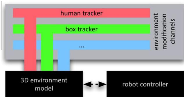
**Fig. 6.** The internal 3D environment model used in the collision avoidance module of the robot controller listens to all communication channels that provide information about modifications in the workspace of the robot.
