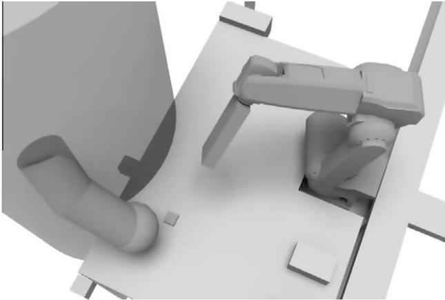
**Fig. 5.** Internal 3D environment model used in the collision avoidance module of the robot controller to compute distances and virtual forces that repel the robot. The cylindrical shape approximates the human co-worker.
