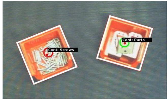
**Fig. 4.** Result of the box tracking module: two red boxes are tracked. Each box is enclosed with a colored rectangle. The center of gravity is calculated for each box and drawn as a dot in the corresponding box color. Additionally, the tracking ids are indicated with colored circles. The content of each tracked box is depicted as a label. (For interpretation of the references to colour in this figure legend, the reader is referred to the web version of this article.)
