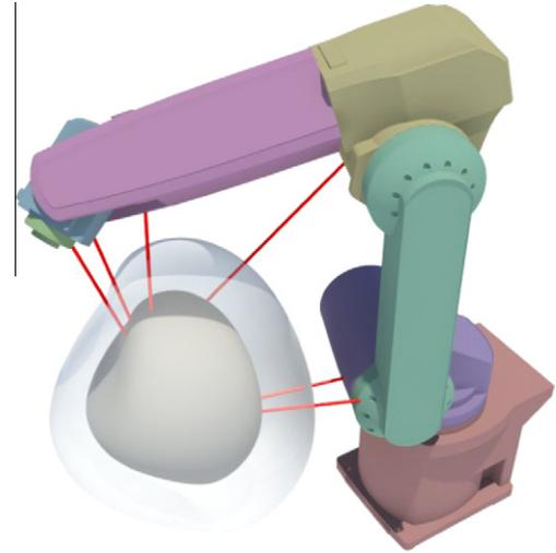
**Fig. 7.** Computing the repelling forces of an obstacle: The red lines illustrate the minimum distances of an obstacle to the body parts of the robot in a given joint configuration. If a distance is below a chosen security threshold (transparent bubble), the distance is used to compute virtual forces on the robot using potential fields. (For interpretation of the references to colour in this figure legend, the reader is referred to the web version of this article.)
