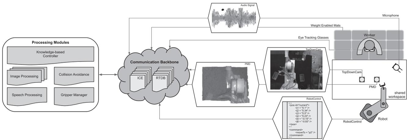
Fig. 3. Schematic overview of applied multi-modal system architecture (left to right): processing module, communication backbone, sensors and actuators, shared workspace.
