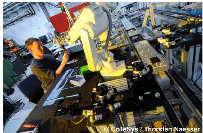
Fig. 1. Hybrid assembly station: human worker drilling together with industrial robot.
