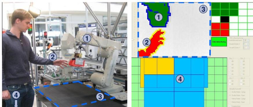
Fig. 8. Safety system in real production cell (left) and segmentation of human and robot based on depth image acquired by PMD camera above workbench (right).
