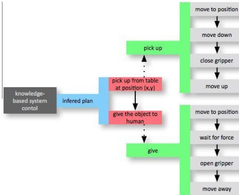
Fig. 9. How inferred plans lead to a robot motion.
