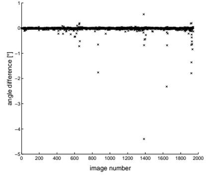
Fig. 14. This plot shows the difference between the  $Z_\infty$  and SSVL rotation estimates along the Y-axis. Only a few outliers can be identified, which are detected by the SSVL's M-estimator. Hence, they do not have any effect on the final result.
