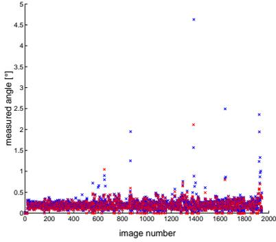
Fig. 13. This figure shows the angles computed for each frame - red the  $Z_\infty$  and blue the SSVL results. The crosses mark the angle about the Y-axis. Only these marks can be identified in the plot.
