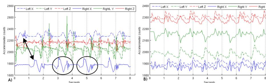
Figure 1 - Output from the GT3X sensors. a) leg sensors; b) arm sensors. Dotted: Left sensor. Full: Right sensor. Blue: X-axis. Green: Y-axis. Red: Z-axis. Arrow shows time shift. Circles show step pattern.
