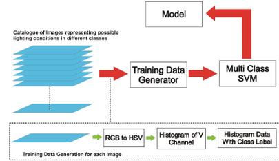
Figure 3: Building blocks of the SVM trainer for lighting conditions
