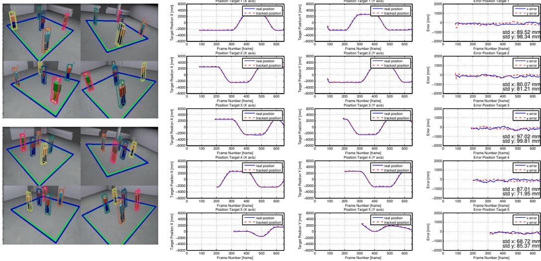
Figure 10: Illustration of the tracking system with 5 targets in the scene moving close to each other and two targets having similar appearance.
