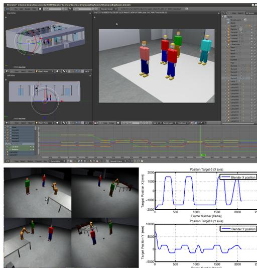
Figure 9: The lab environment modelled in 3D and extraction of simulated trajectory data.
