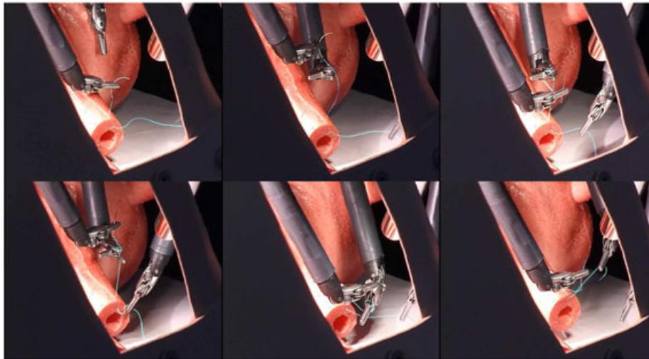
Figure 12. Subsequent stages of the knot-tying process during one user demonstration
