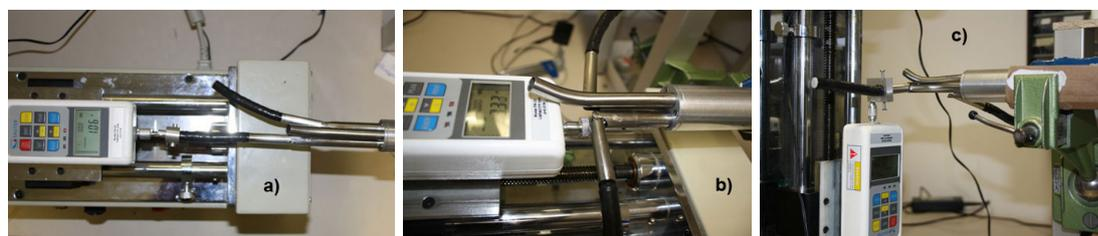
**Figure 6.9:** Linear force measurement of the prismatic joint and torque measurement of the rotational joint: a) pulling in straight form b) pushing with the upper-arm tube c) rotation force at the wrist
