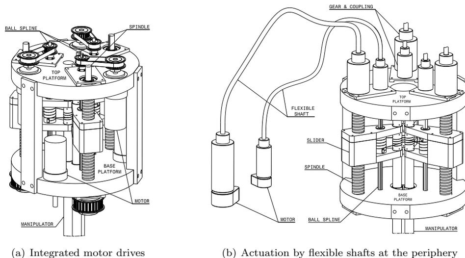
**Figure 4.7:** Concepts of the linear and rotary joint of the manipulators: a) Direct drive by motors integrated into the platform b) Actuation of the passive platform mechanism by using flexible shafts.
