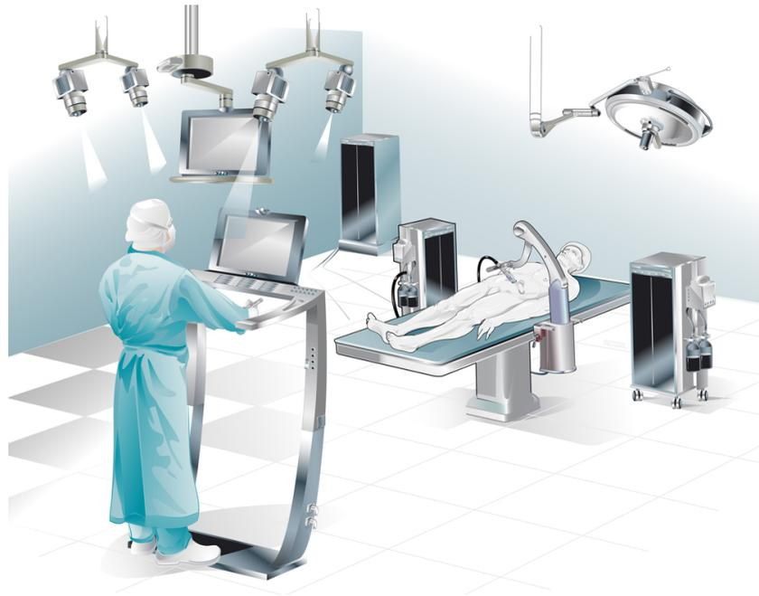
**Figure 1.1:** Vision of the single-port system: The intuitive master console on the surgeon's side and the guiding manipulator with the single-port platform on the patient's side (MITI, Klinikum rechts der Isar, Germany).
