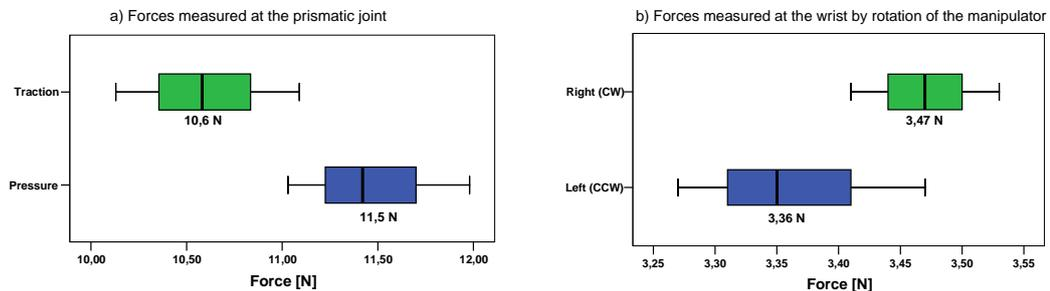
**Figure 6.13:** Results of the measured forces with the prismatic and rotational joints
