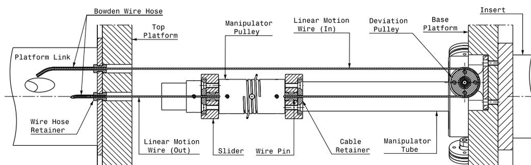
**Figure 4.13:** Sectional view illustrating the linear actuation mechanism of the manipulator
