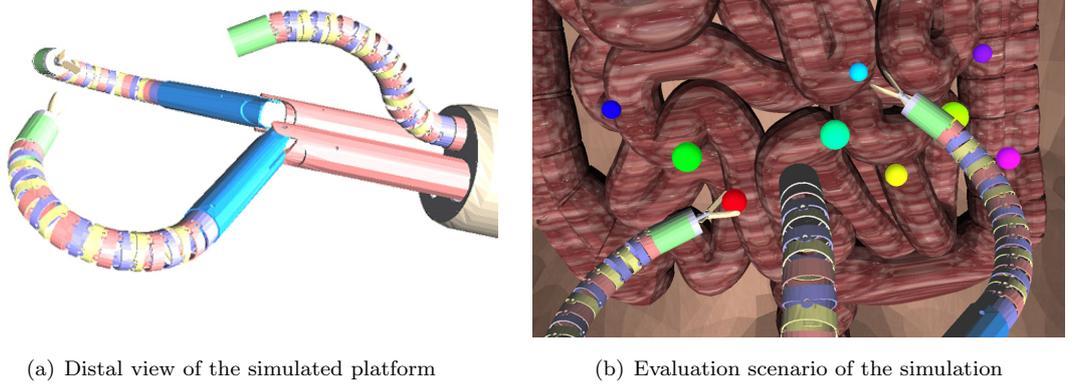
**Figure 5.7:** Simulation environment for the evaluation of the platform and the kinematics.
