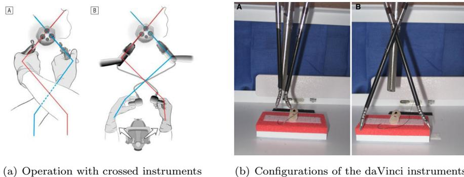
**Figure 3.2:** Current approaches for single-port surgery: a) Comparison of the conventional (A) and robotic (B) single-port surgery b) Standard (A) and chopstick setup (B) of the daVinci instruments [104, 105]
