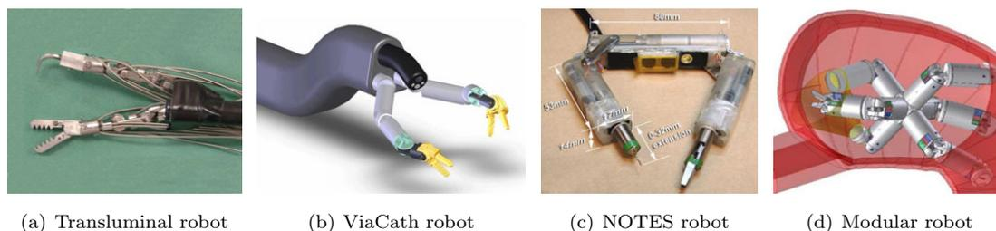
**Figure 2.6:** Design of transluminal robots: a) Transluminal endoscopic robot [131] b) ViaCath endoluminal robot [132] c) Miniature NOTES robot [133] d) Reconfigurable modular endoluminal robot [134]
