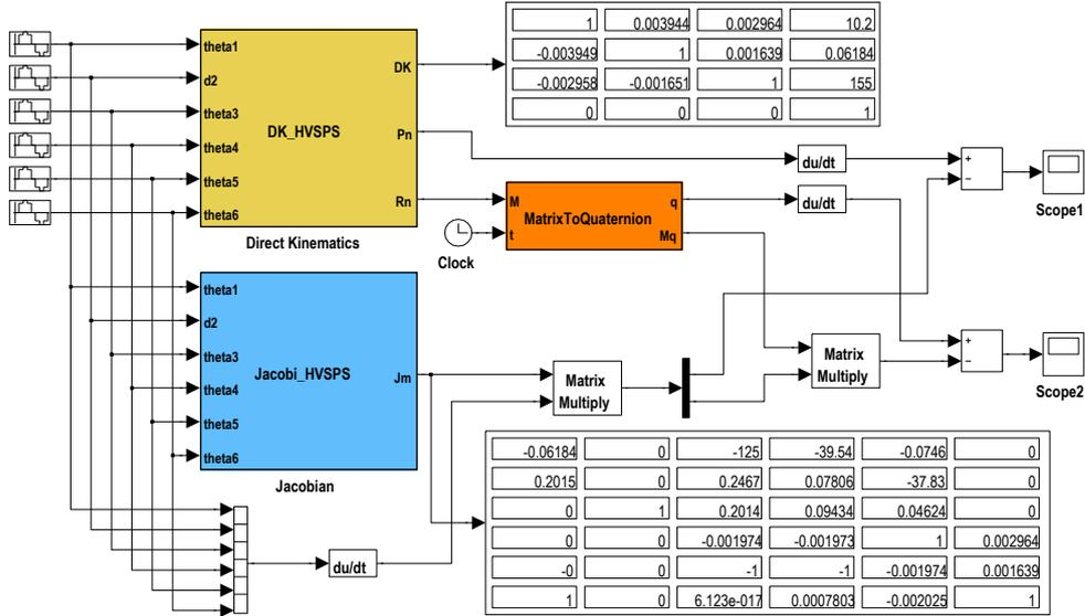
**Figure 5.4:** Matlab-Simulink program for the numeric verification of the Jacobian. DK\_HVSPS computes the forward kinematics and Jacobi\_HVSPS the Jacobian of the manipulator. In MatrixToQuaternion, the quaternions  $q$  and the matrix  $M_q$  are determined from the rotation matrix  $R_e$
