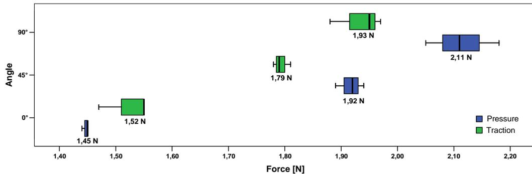
Figure 6.10: Results of the force measurements by horizontal deflection of the bending section
