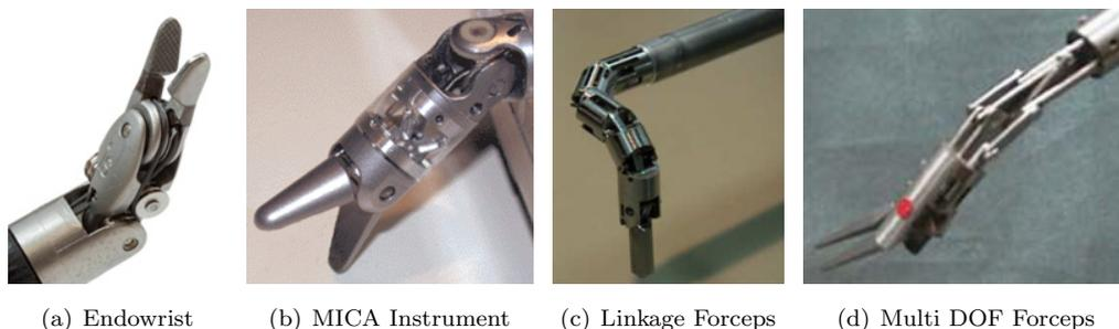
**Figure 2.1:** Instruments with additional articulations: a) Endowrist Instrument [24] b) MICA Instrument [76] c) Hand-held multi-slider linkage forceps [63] d) Link driven multiple DOF forceps [40]
