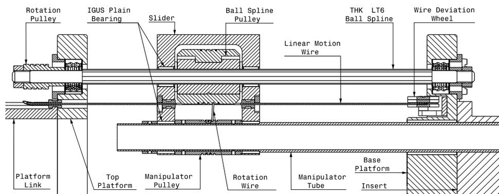
**Figure 4.10:** Sectional view of the linear and rotary actuation mechanism of one manipulator.
