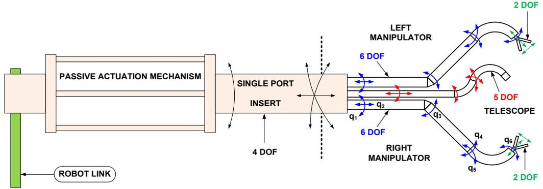
Figure 3.6: Schematic drawing of the semi-rigid single-port surgical platform: Two 6 DOF manipulators ( $\emptyset 12\text{mm}$ ), a 5 DOF flexible telescope ( $\emptyset 10\text{mm}$ ) and a 4 DOF robot guiding the insert ( $\emptyset 34\text{mm}$ ).
