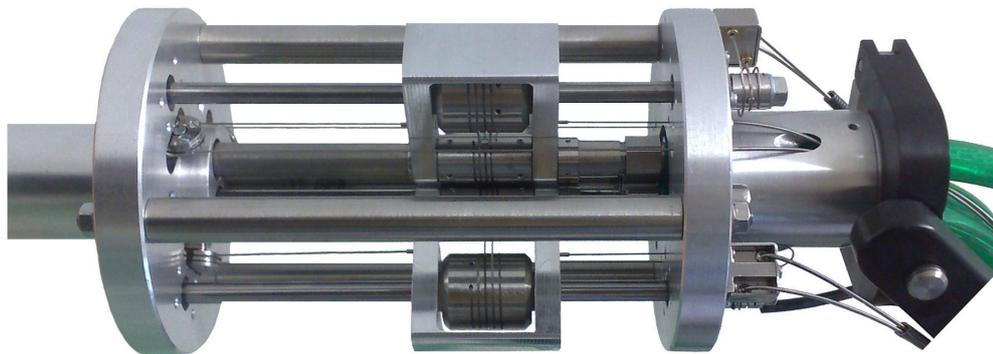
**Figure 4.9:** Proximal unit of the developed single-port platform including the linear and rotary articulations as well as the linkage for the guiding system.
