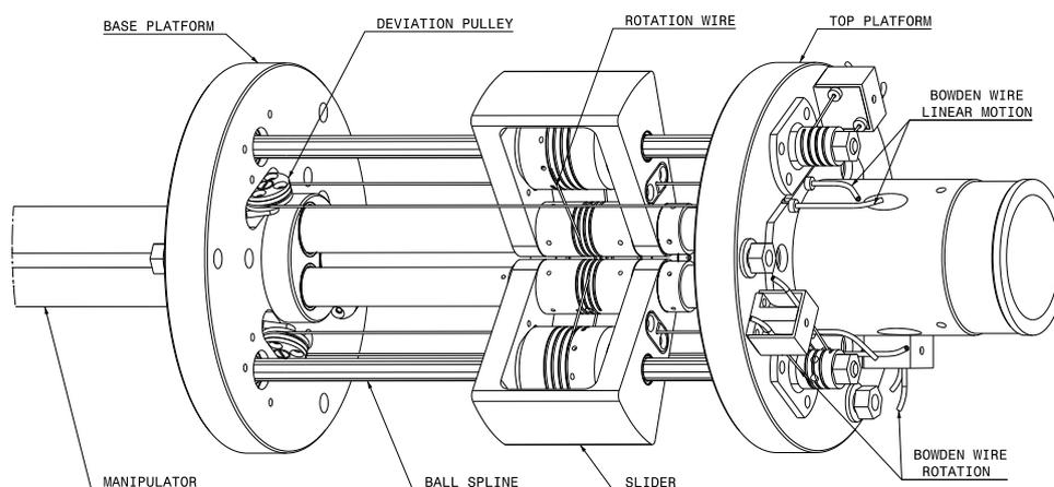
**Figure 4.8:** Concept of the linear and rotary joint actuation by using bowden wire mechanism.
