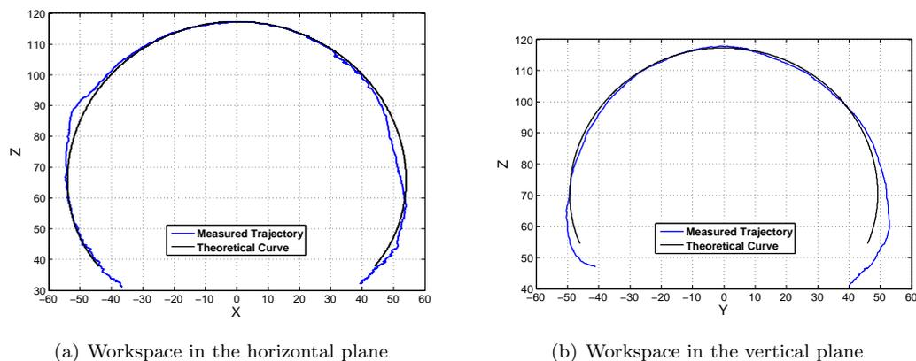
**Figure 6.3:** Measured workspace of the bending section in the horizontal and vertical planes.
