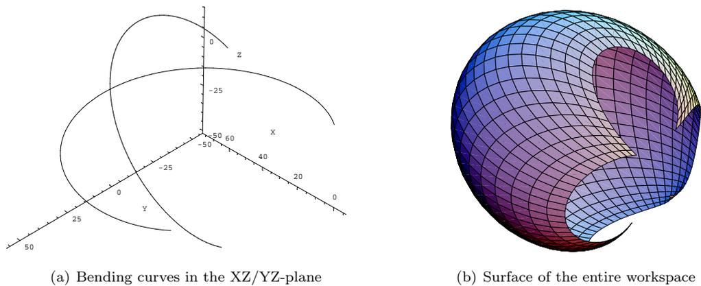
**Figure 6.2:** Theoretical workspace of the gastroscope bending section.
