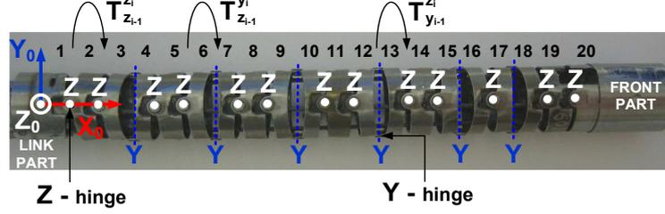
**Figure 5.2:** Bending section of the Karl-Storz gastroscope illustrating the configuration of the hinges and their orientations. The bending section comprises the three different “passive” joints  $T_{zz}$ ,  $T_{yz}$  and  $T_{zy}$ .
