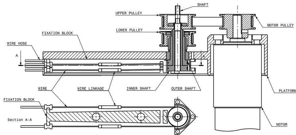
**Figure 4.18:** Sectional view of the drive unit and bowden wire mechanism for distal articulations
