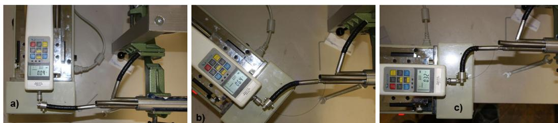
**Figure 6.7:** Measurement of the forces applied by the bending section on the manipulator tip at different bending angles of the deflecting: a) straight configuration b) deflecting at  $45^\circ$  c) deflecting at  $90^\circ$
