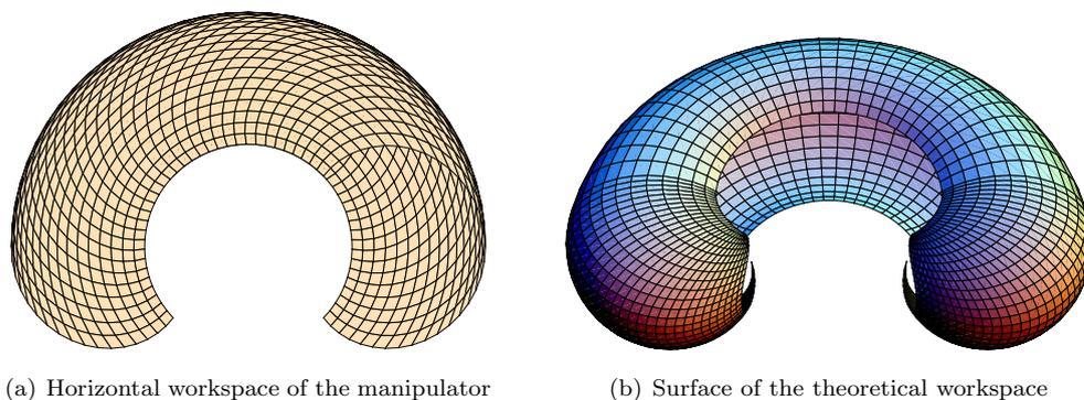
**Figure 6.4:** Surfaces of the theoretical workspace of the manipulator determined with the kinematics
