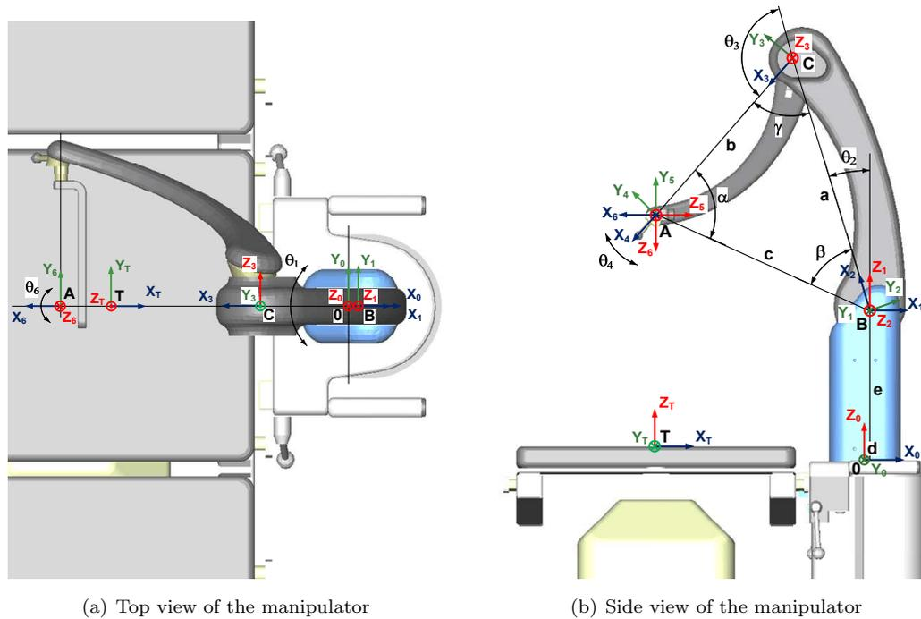
**Figure A.1:** Design of the SoloAssist telemanipulator attached to the operating table. All the joints and frames are indicated and labeled.
