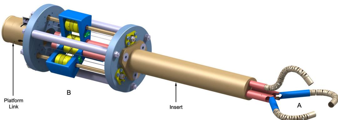
**Figure 4.1:** Design of the highly versatile single-port platform. A: Distal dexterity inside the body. B: Actuation mechanism for rotation and linear motion ( $\varnothing 100 \times 160\text{mm}$ )
