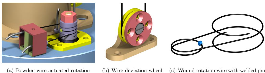
**Figure 4.12:** Detailed views of the wire actuation: a) Design of the drive transmission to the ball spline shaft b) Design of the wire deviation wheel c) Wound wire for the rotation transmission to the manipulator
