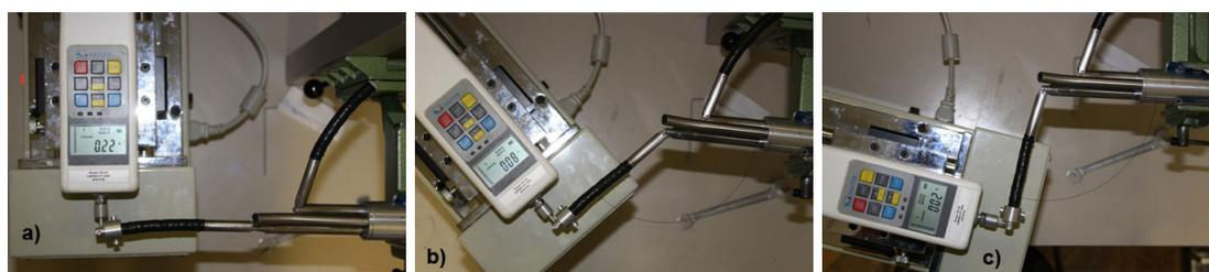
**Figure 6.8:** Measurement of the forces applied by the elbow joint on the manipulator tip at different bending angles of the elbow joint: a) straight configuration b) elbow bent to  $50^\circ$  c) elbow bent to  $80^\circ$
