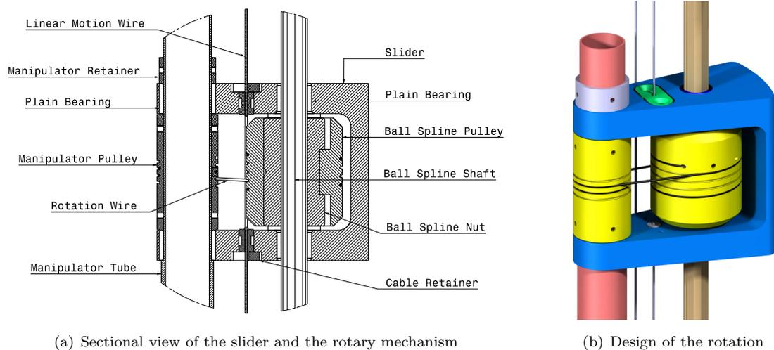
**Figure 4.11:** Design of the rotation mechanism: a) Sectional view illustrating the implemented components b) 3D view of the rotation mechanism of one manipulator
