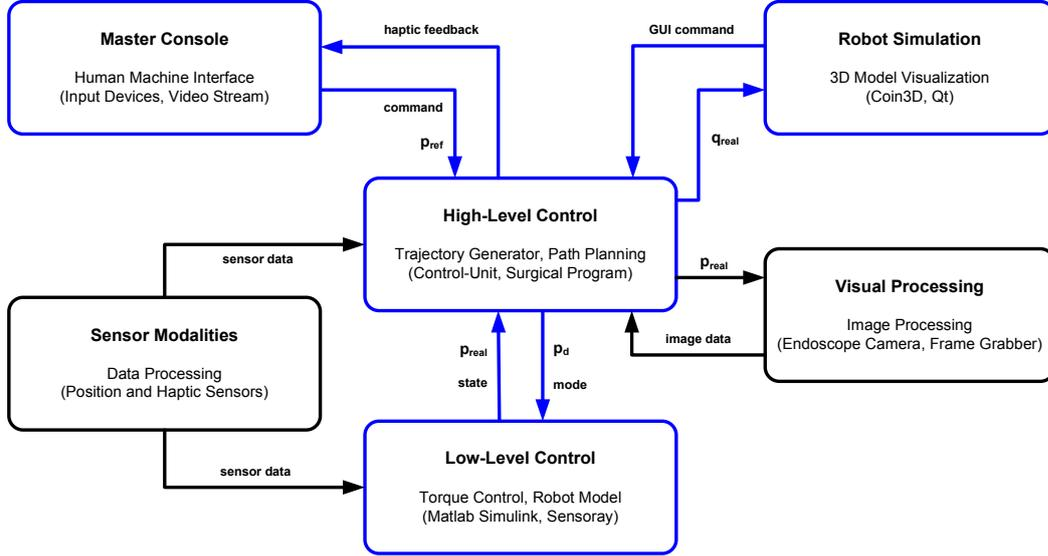
**Figure 5.1:** Concept of the control architecture for the single-port system. The high-level control forms the central control unit for all the modules. The provided and required interfaces  $p_{ref}$ ,  $p_d$  and  $p_{real}$  are the reference, desired and real tool positions.
