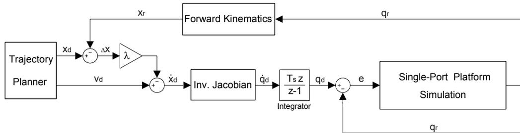
**Figure 5.8:** Velocity-based control of the single-port manipulator. A basic velocity profile is used to control the simulation of the platform.
