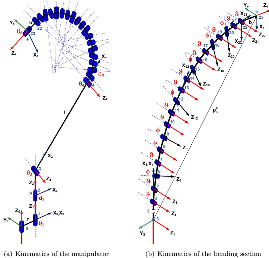
**Figure 5.3:** Schematic drawing of the manipulator and the bendable section kinematics generated with the robotic toolbox in Matlab [146]. It illustrates the individual joints and the used coordinate axis.
