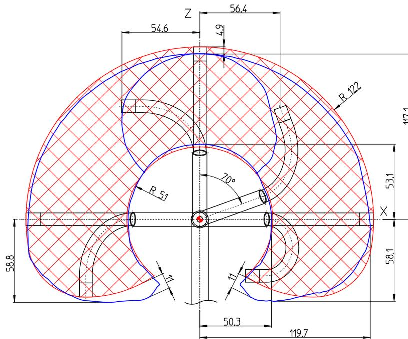
**Figure 6.5:** Workspace evaluation of the distal dexterity of the manipulator in the horizontal plane: Red hatched surface presents the theoretical workspace and the blue lines present the measured trajectories.
