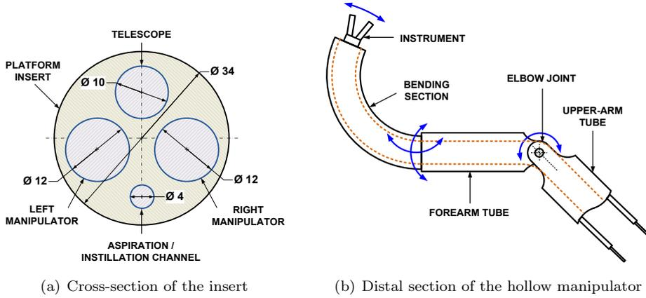
**Figure 3.7:** a) Cross-section of the insert with the configuration of the manipulators and the telescope
