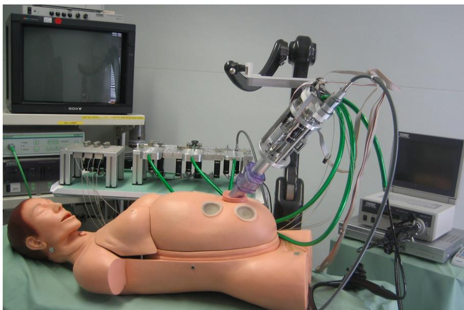
**Figure 4.2:** The overall highly versatile single-port system: Passive platform attached to the SoloAssist guiding system and actuated by the active drive unit at the periphery.
