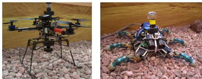
(a) flying robot with a catadioptric (b) crawling robot with a catadioptric (up) and fisheye (down) camera camera
